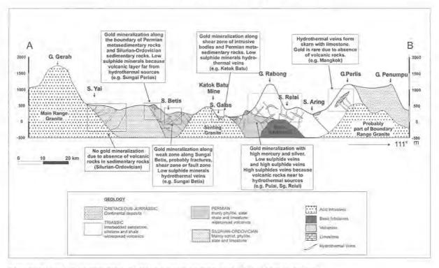
Figure 3: Gold mineralization model for cross section A-B, at southern Kelantan.
