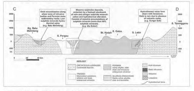
Figure 4: Gold mineralization model for cross section C-D, at northern Kelantan.
