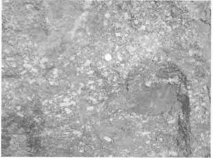
**Figure 5:** End stages of K-feldspar dispersion in the gabbroic rock. In this stage the euhedral K-feldspar forms a schlieren–like texture in gabbroic
