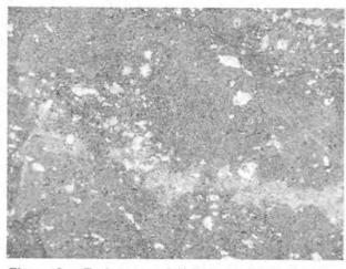
Figure 6: : End stages of K-feldspar dispersion in the gabbroic rock. Note the various sizes of the K - feldspar crystals.
