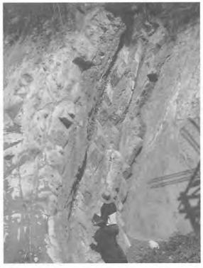
Figure 5. Grade III to IV sandstone and shale of the weathering profiles (Location: Survey Hypermarket, Likas)
