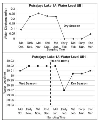
**Figure 2.** Graph of water level and water discharge for UB1 wetland cell from mid October 2001 to end March 2002.
