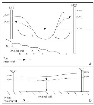
**Figure 6.** Schematic hydrogeological section of a) Sg. Chuau and b) Sg. Bisa (river was dry).
