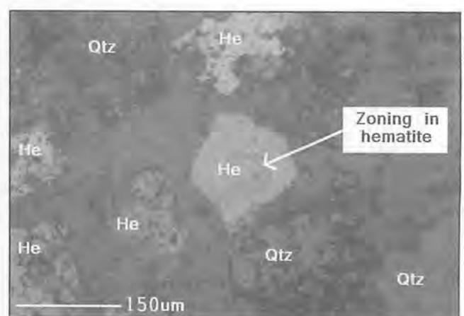
Figure 3. Replacement zoning in hematite (He) grain. Also present are quartz (Qtz) grains. Rahman Hydraulic Mine, Klian Intan. Plane polarised light.
