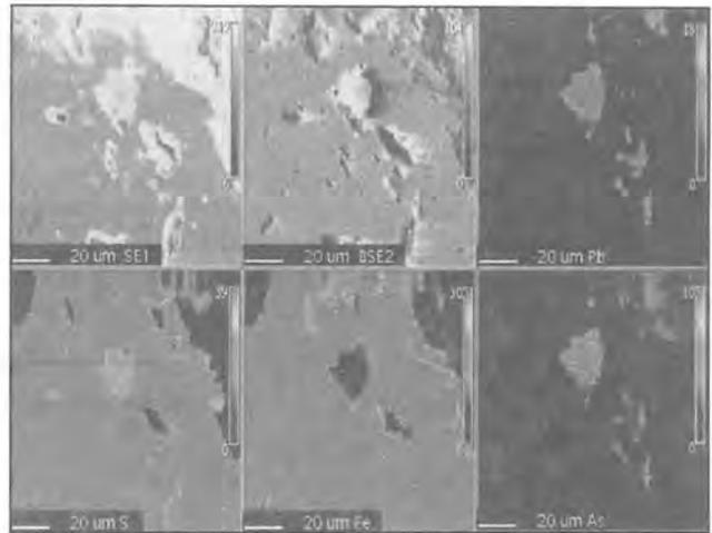
**Figure 7.** X-ray map showing tsugaruite ( $Pb_7As_2S_7$ ) present as inclusions in pyrite ( $FeS_2$ ). Pyrite is the dominant mineral here. Rahman Hydraulic Mine, Klian Intan.
