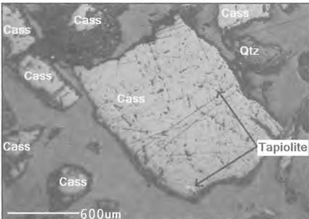
**Figure 5.** Exsolutions of tapiolite in cassiterite (Cass). Also present are quartz (Qtz) grains. Rahman Hydraulic Mine, Klian Intan. Plane polarised light.
