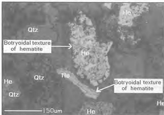
Figure 2. Polished section sample shows botryoidal texture in hematite (He) grains. Also present are quartz (Qtz) grains. Rahman Hydraulic Tin Mine, Klian Intan. Plane polarised light.
