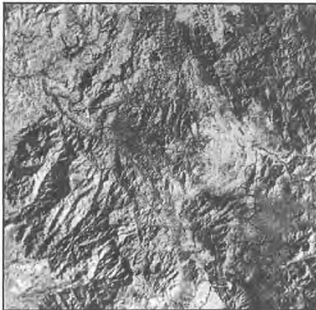
Figure 2. Linear contrast stretched of Landsat MSS band 7 of the Upper Perak Valley area. The image is found best particularly for lineament mapping compared to other images.
