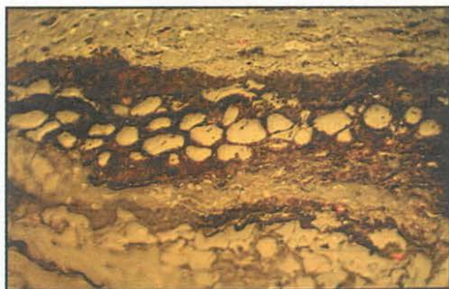
Figure 6. Accumulation of disordered suberinite forms bituminite (dark brown amorphous mass) seen here surrounding phlobaphinite bodies that have softened and swollen as a consequence of plastic deformation; reflected light, oil immersion, field width = 0.2 mm.
