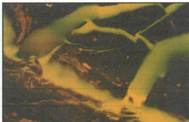
Figure 7. Exsudatinite exerting pressure upon the release of hydrocarbon material forming a network that caused the coal to fracture; blue light excitation, field width = 0.2 mm.
