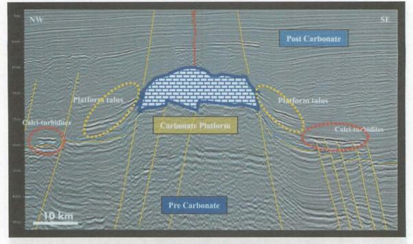
Figure 5. A seismic line across the carbonate high showing carbonate talus scree and turbidite fans.
