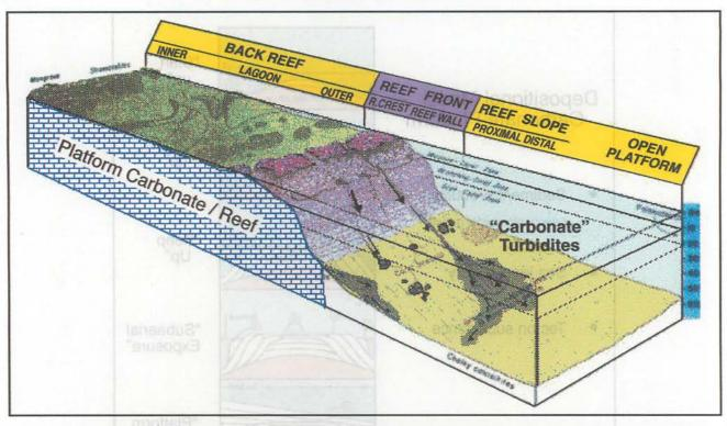
Figure 9. Carbonate turbidite depositional model: Central Luconia rimmed platform.
