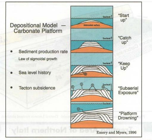
Figure 7. Schematic model for an isolated carbonate platform.
