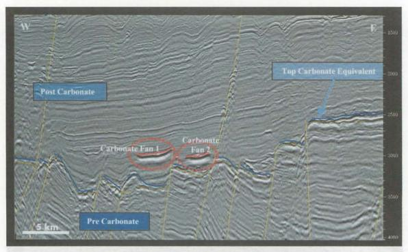
Figure 6. A seismic line across the distal turbidite fans.
