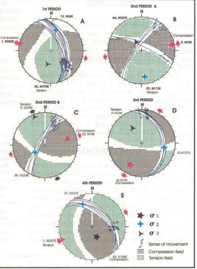
**Figure 11**. Palaeostresses and stress field related to the deformation of the Kenerong Leucogranite at Sungai Renyok, Jeli, Kelantan. A) First period; B) Second period A; C) Second period B; D) Third period; and E) Fourth period.
