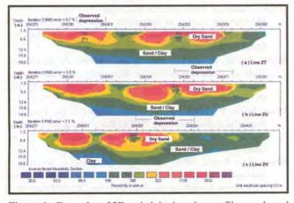
Figure 6. Examples of 2D resistivity imaging profiles conducted in the study area.
