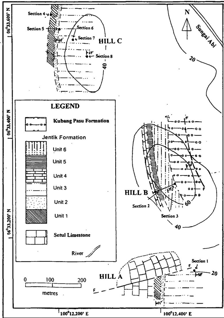
Figure 3. Outcrop geological map of Guar Sanai and logged section location.
