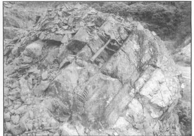
Figure 7. Calcareous sandstone bed (where the hammer is placed) on top of a sequence of thin to moderately bedded sandstone.
