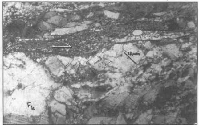
Figure 4. Photomicrograph of kinked feldspar (Fk) and displaced broken feldspar (shown by thin half arrow) due to dextral movement (thick half arrow) (after Zaiton Harun (1994).
