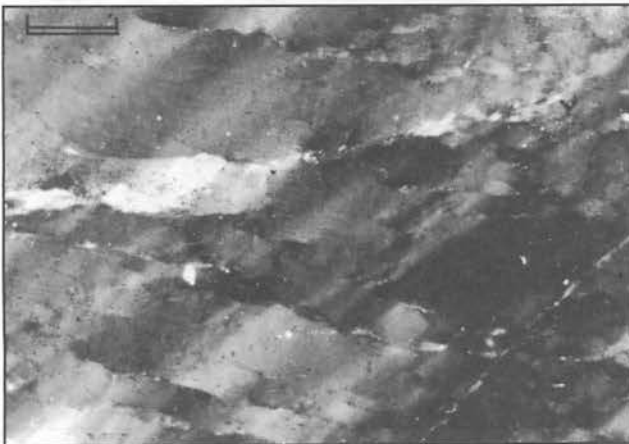
Figure 3. Patchy extinction (mosaicism) and cleavage in ESE direction are evidence for shock metamorphism. Thin section of vein quartz cut from a sill-dyke stock work in Carboniferous Singa beds, Sungai Batu Asah, Pulau Langkawi. Part-polarised light. Bar is 100 microns.
