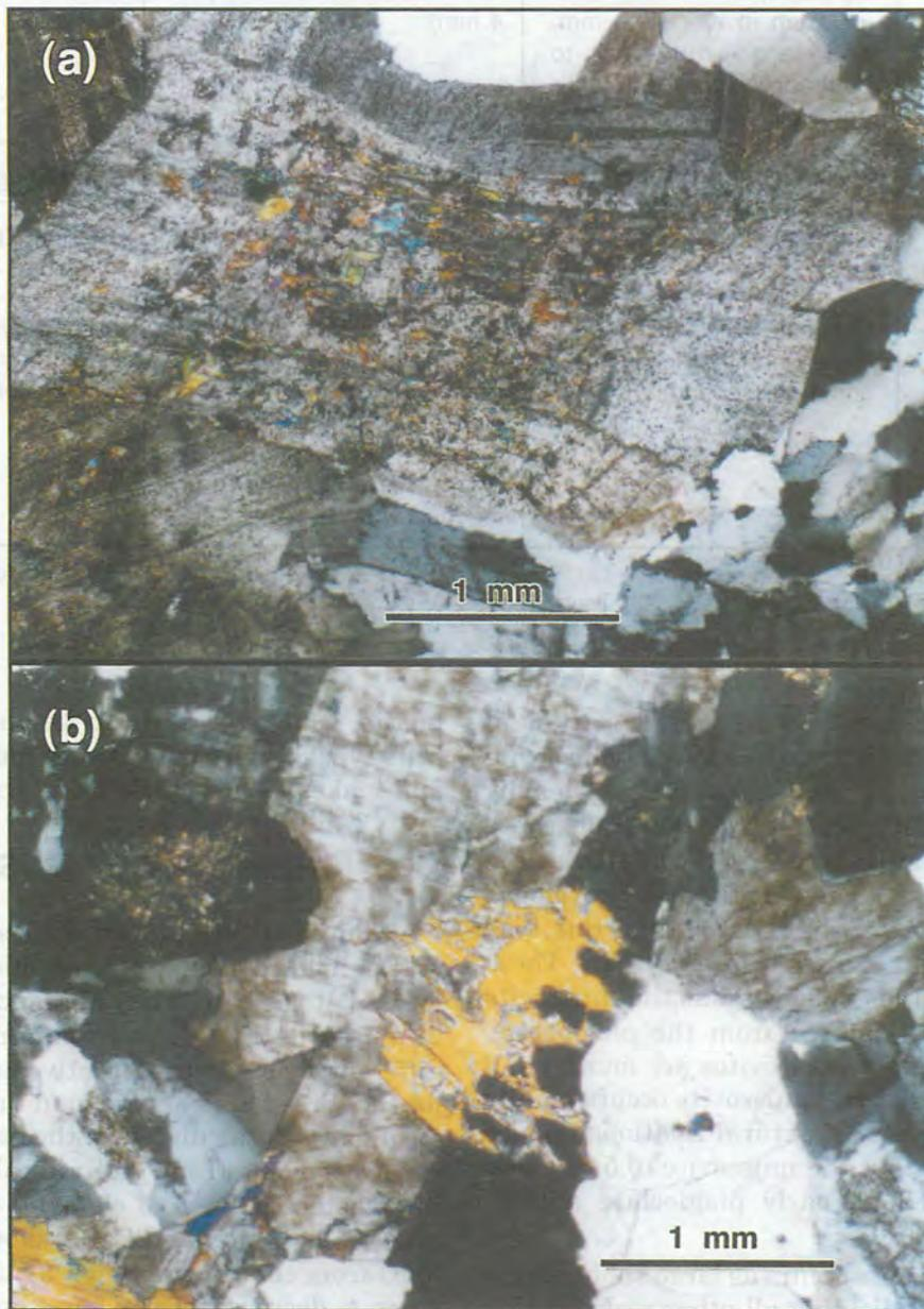
**Figure 2.** (a) Fine grained muscovite associated with sericite in the plagioclase crystal (sample: DBMG) (scale bar = 1 mm). (b) Skeletal muscovite in the K feldspar (sample: DBMG) (scale bar = 1 mm).
