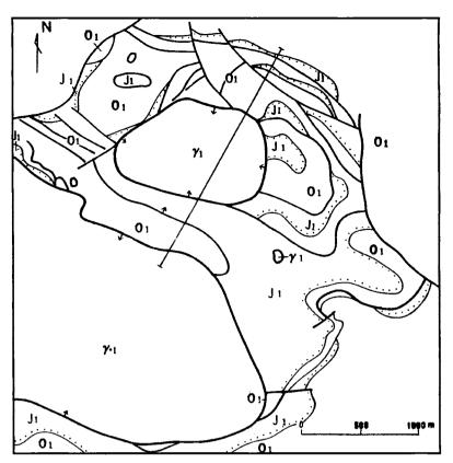
**Figure 3.** Nappe structures of the Shansonggang coal mining area (after Mang, 1986, revised).  $\gamma_1$  – Archaeozoic migmatite;  $O_1$  – Early Ordovician limestone;  $J_1$  – Early Jurassic coal-bearing strata;  $\gamma_1 = \gamma_2 = -$  Fault and its dip;  $\mu_1 = -$  section line.
