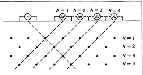
**Figure 2.** The presentation of dipole-dipole resistivity results on a pseudosection. 'N' represents the relative spacing between the current and potential electrode pairs.
