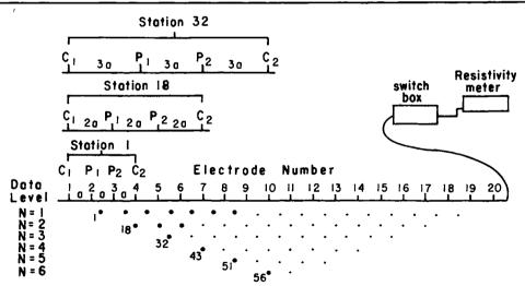
**Figure 3.** The arrangement of electrodes for 2-D electrical imaging survey and the sequence of measurements used to build up a pseudosection.
