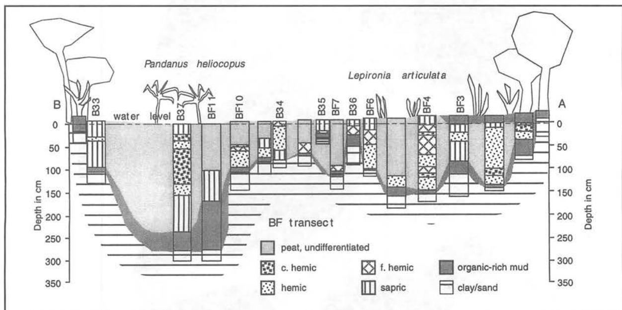
**Figure 8.** Cross-section of the traverse BF showing peat stratigraphy and peat thickness variation in the southern littoral part of Tasik Bera. The distance A to B is 1,000 m.
