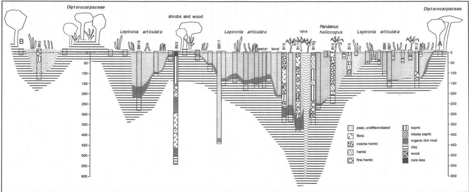
Figure 10. Cross-section of the traverse BB showing peat stratigraphy and peat thickness variation in the northern littoral part of Tasik Bera. The distance A to B is 3,000 m.
