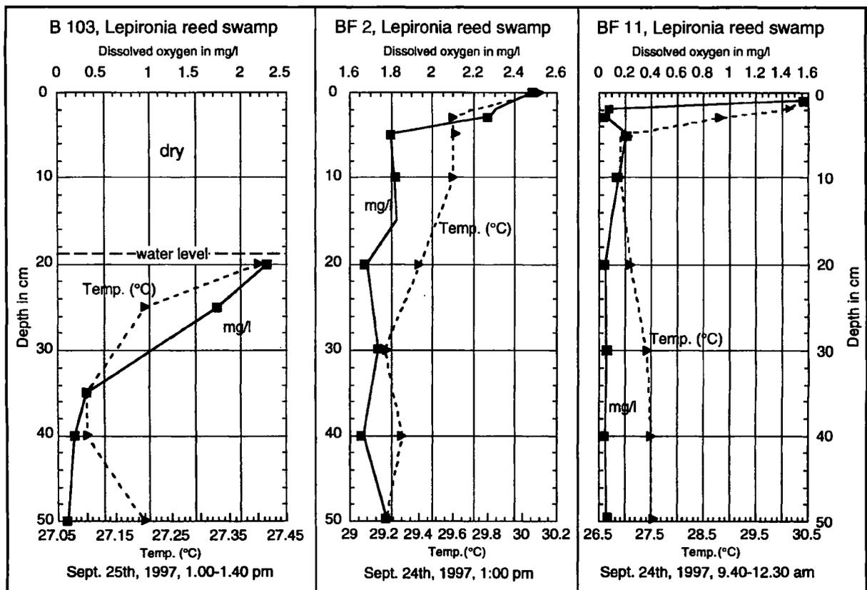
Figure 6. Dissolved oxygen measurements along the transect BF (3°04.500'N).
