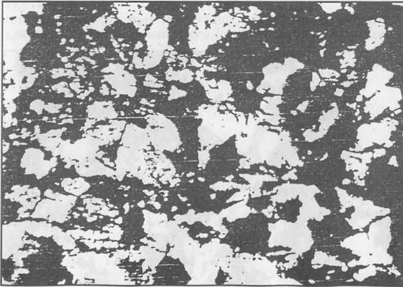
**Figure 15.** Diffusing and penetrating deformation. III05, stable sliding, 200 Mpa, 500°C, x40, (+).
