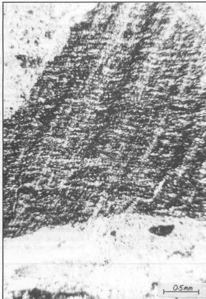
Figure 16. Photomicrograph showing flow texture within the ultramylonite resulting from the first ductile deformation (x-nicols).
