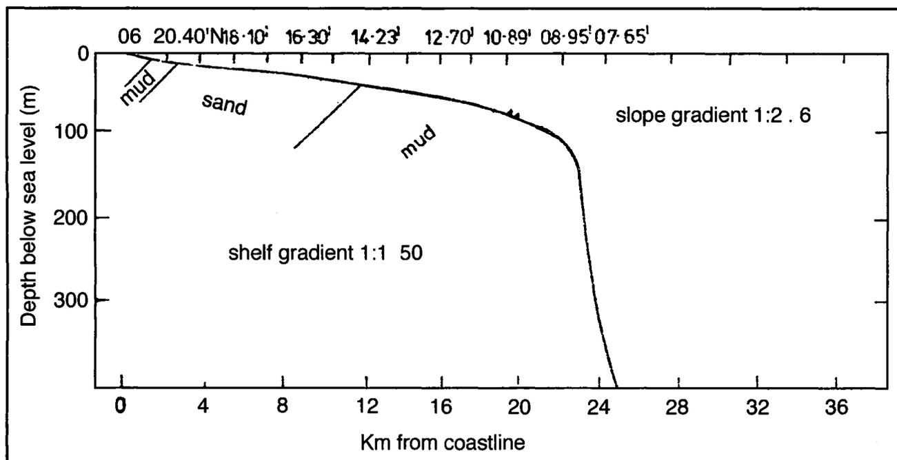
Figure 3. Echo sounder profile near Badagry (long 03°02'04"E) showing shelf morphology and sediment outcrops.
