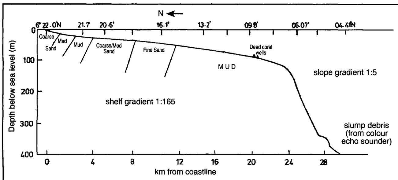
Figure 4. Echo sounder profile off Lagos (long 03°35'0"E) showing shelf morphology and sediment outcrops.
