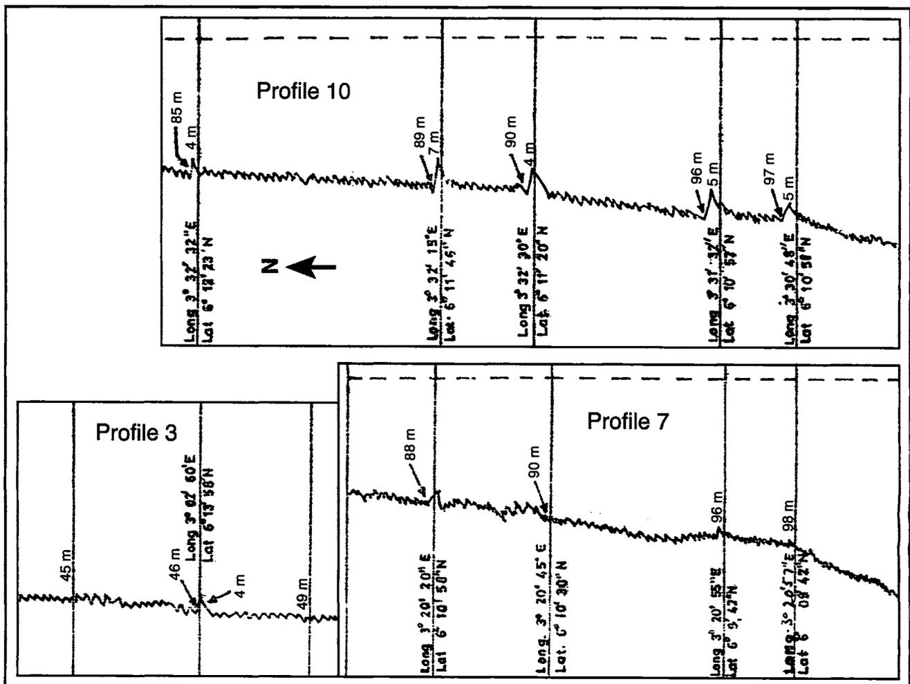
Figure 7. Echo profiles along lines 3, 7 and 10 showing positions of coral banks (modified after Awosika, 1990).
