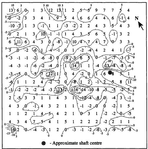
Figure 11. Magnetometer readings with detector at 110 cm height with 2 m grid in locating shaft 4a. Contour interval 5 gamma.
