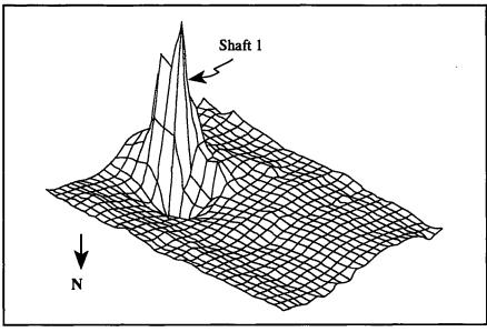
**Figure 4.** A three dimensional plot of anomalies showing the location of shaft 1 over a positive anomaly.
