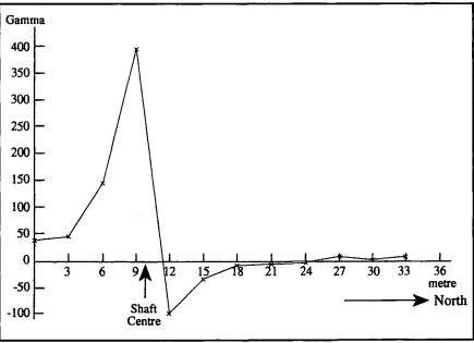
LOCATING ABANDONED MINE SHAFTS USING A PROTON MAGNETOMETER
