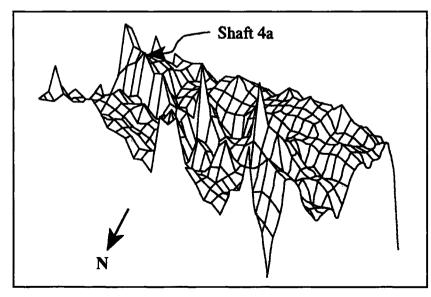
Figure 13. A three dimensional plot of anomalies in 4a square grid. It is a challange to locate a shaft based on anomalies shown.
