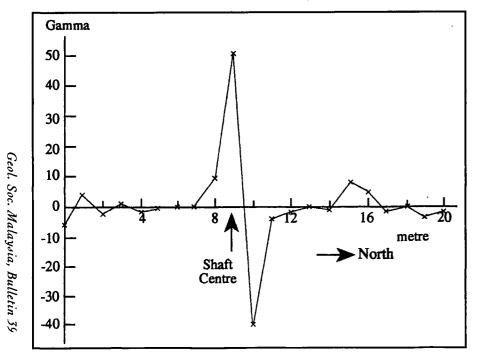
Figure 8. South-North traverse across shaft 4 with detector at 60 cm height.
