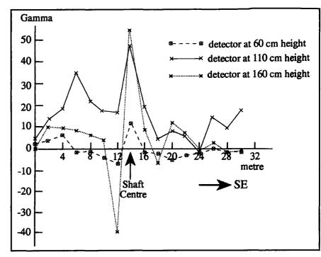
Figure 7. Traverse 8 (NW-SE direction) across a shaft with different detector heights.
