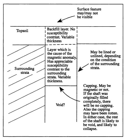
Figure 1. A cross section across a typical abandoned shaft.
