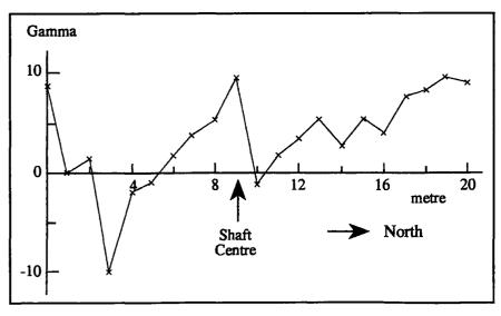
Figure 9. South-North traverse across shaft 7 with detector at 60 cm height.
