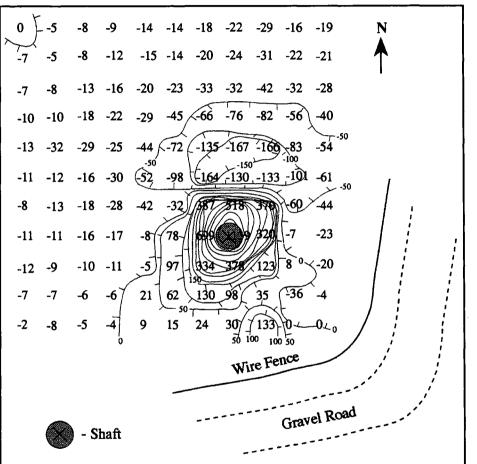
Figure 14. Magnetometer readings with detector at 60 cm height with 2 m grid. Contour interval 50 gamma.
