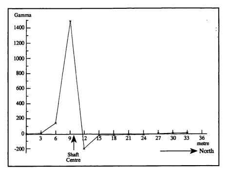
Figure 6. South-North traverse across a shaft with detector at 60 cm height.
