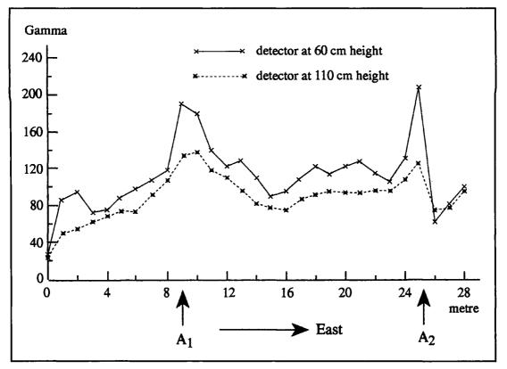
Figure 17. West-East traverses across a stream with detector at 60 and 110 cm heights in Wallsend site.
