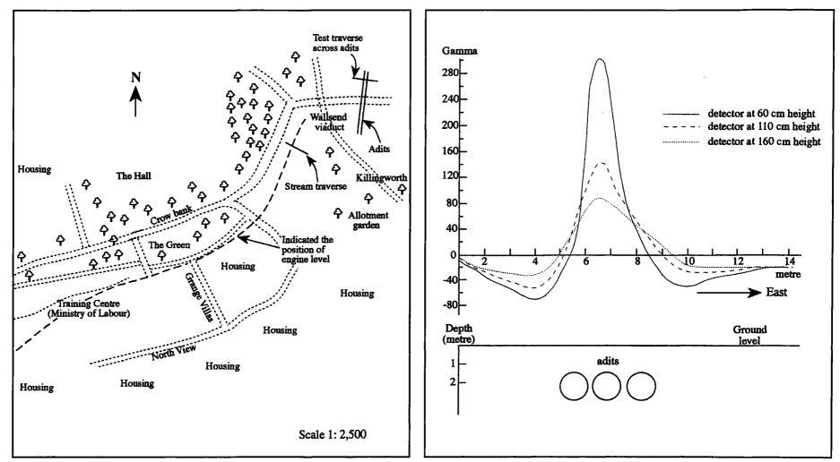
**Figure 15.** The map of the Wallsend site showing the positions of engine level, adits and traverses.
