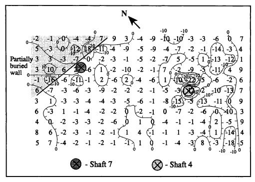
Figure 10. Magnetometer readings with detector at 110 cm height with 3 m grid in locating shafts 4 and 7. Contour interval 10 gamma.
