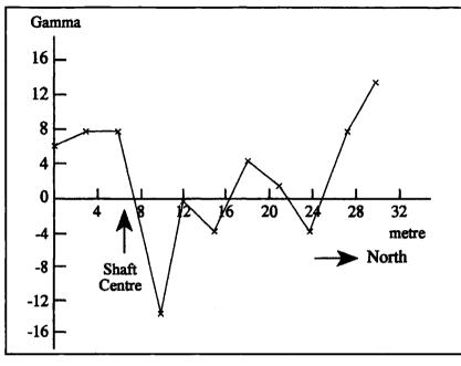
Figure 12. South-North traverse across shaft 4a with detector at 110 cm height.
