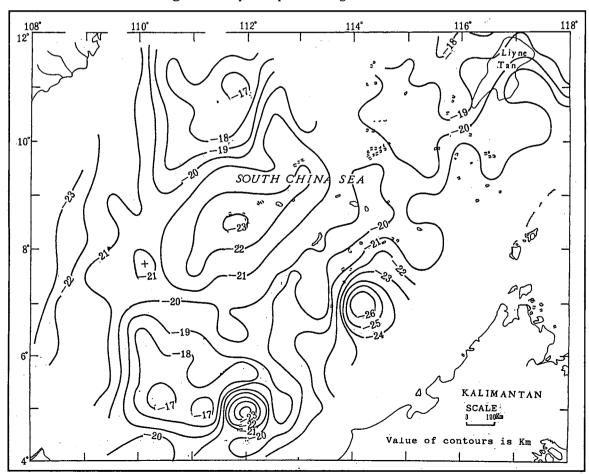
Figure 3. Depth map of the lower surface of magnetic body.
