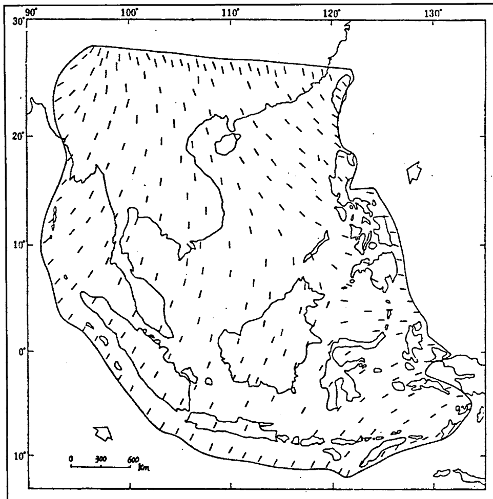
Figure 16. Distribution of maximum compressive principal stress in the Nansha Islands and its vicinity.
