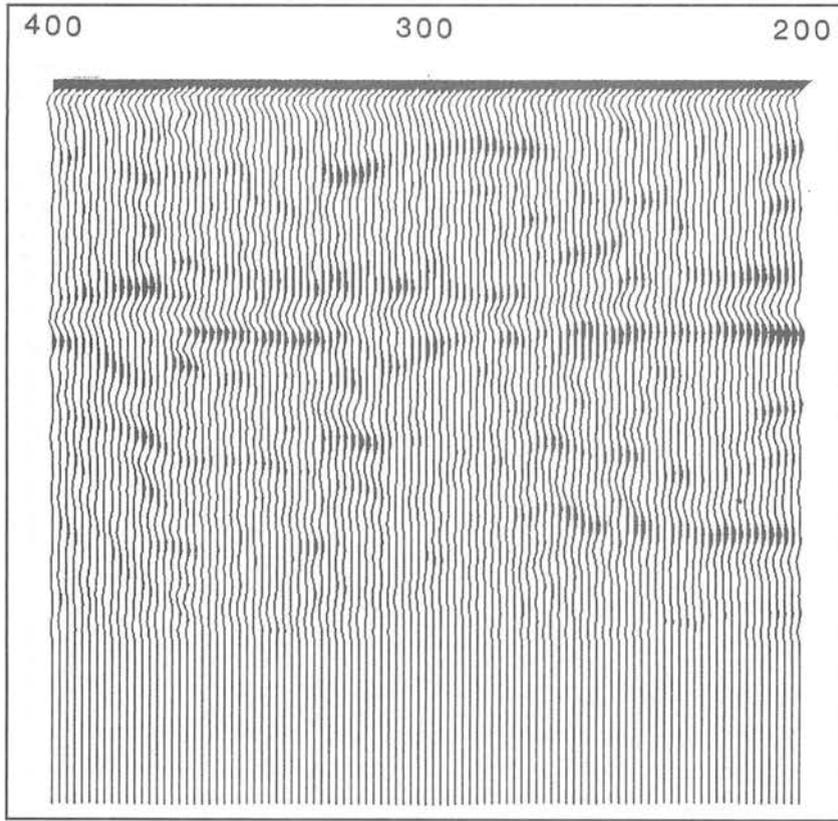
Figure 4. Autocorrelation function of CDP 200 through CDP 400.
