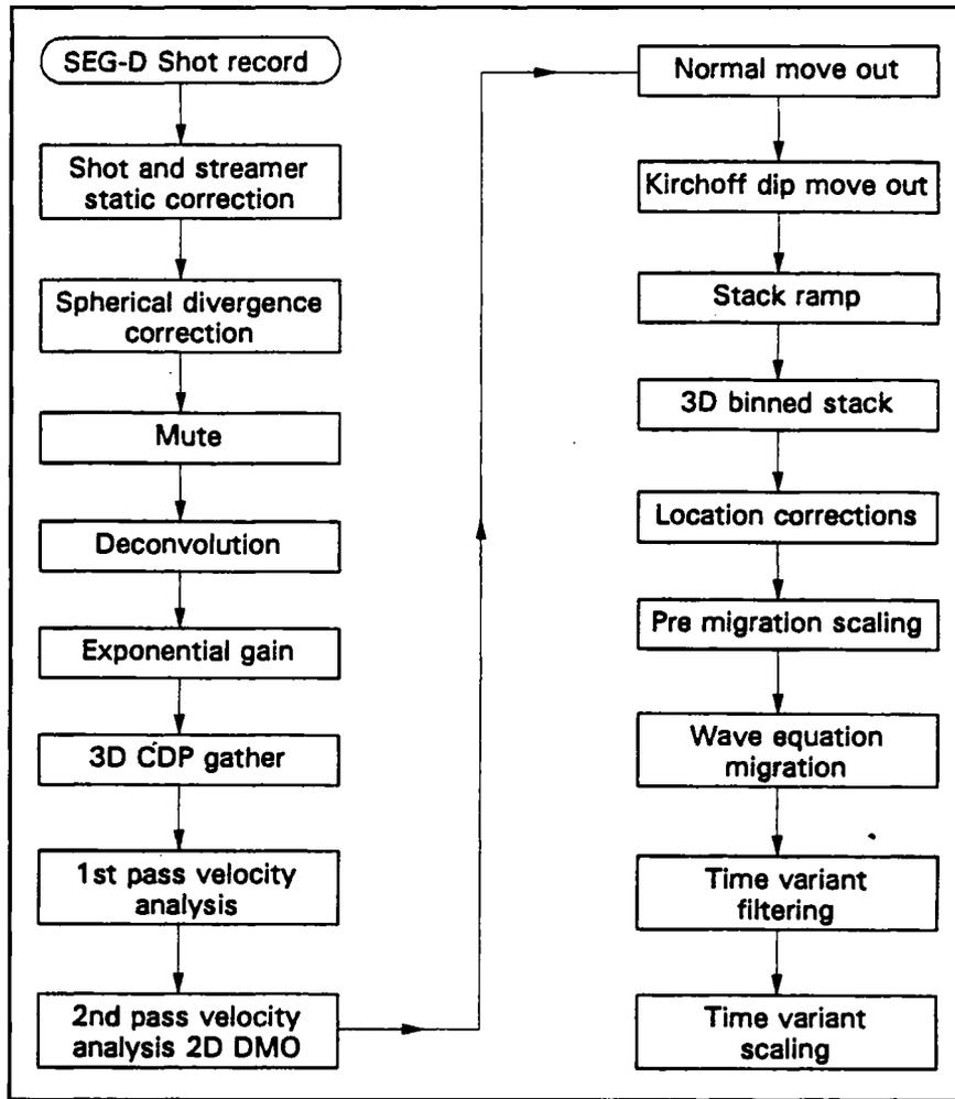
Figure 2. 3-D processing sequence.
