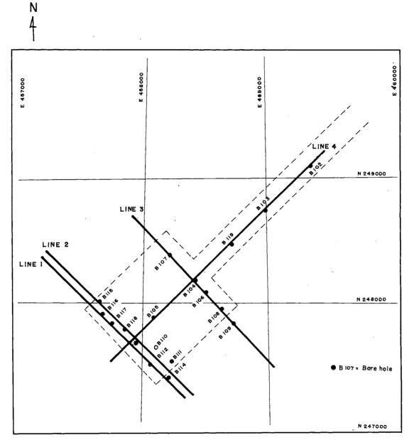
Figure 2. Seismic lines and location of the boreholes.
