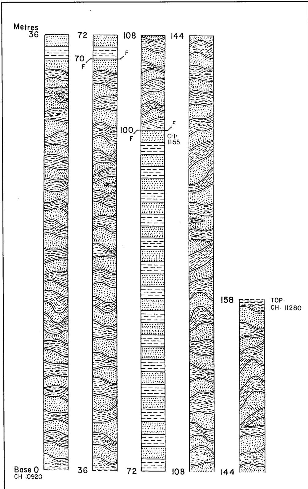
Figure 3. Detailed stratigraphic section recorded at road cut no. 9. For legend see Figure 2.
