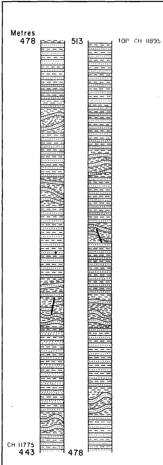
**Figure 4.** Detailed stratigraphic section recorded at road cut no. 8. For legend see Figure 2.
