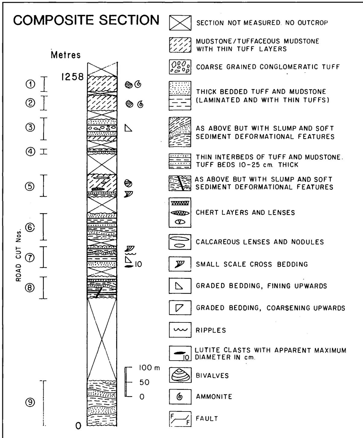
Figure 2. Composite section exposed in the Bypass compiled from road cuts 1-9.
