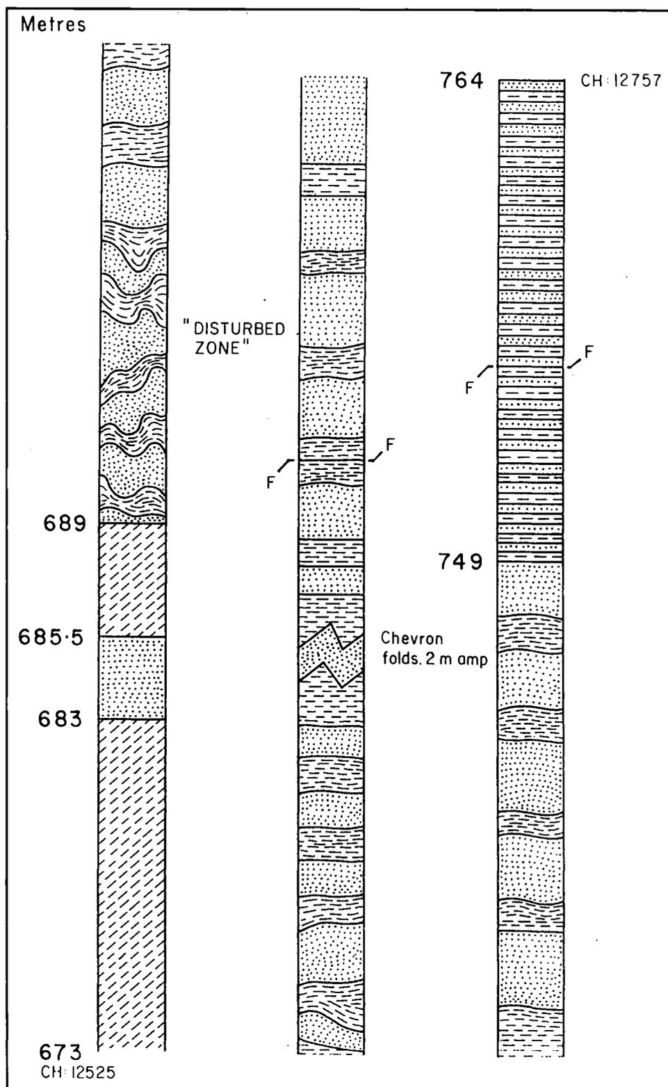
Figure 6. Detailed stratigraphic section recorded at road cut no. 6. For legend see Figure 2.
