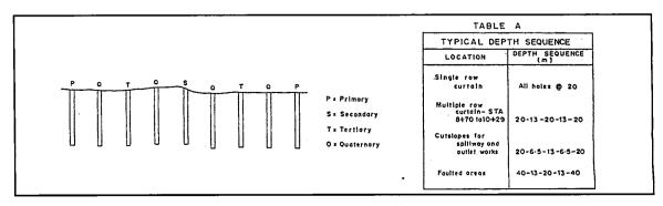
Figure 7. Grouting sequences.
