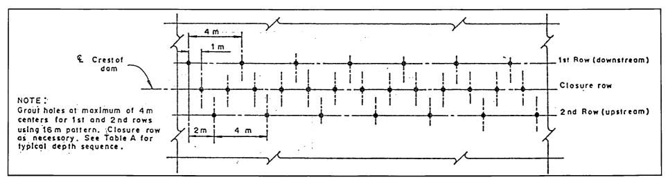
Figure 6. Typical grout hole pattern.
