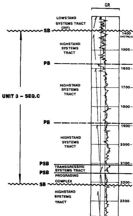
Figure 17. Interpreted systems tracts in neritic-bathyal facies of Unit 3–Seq. C at well No: 8.
