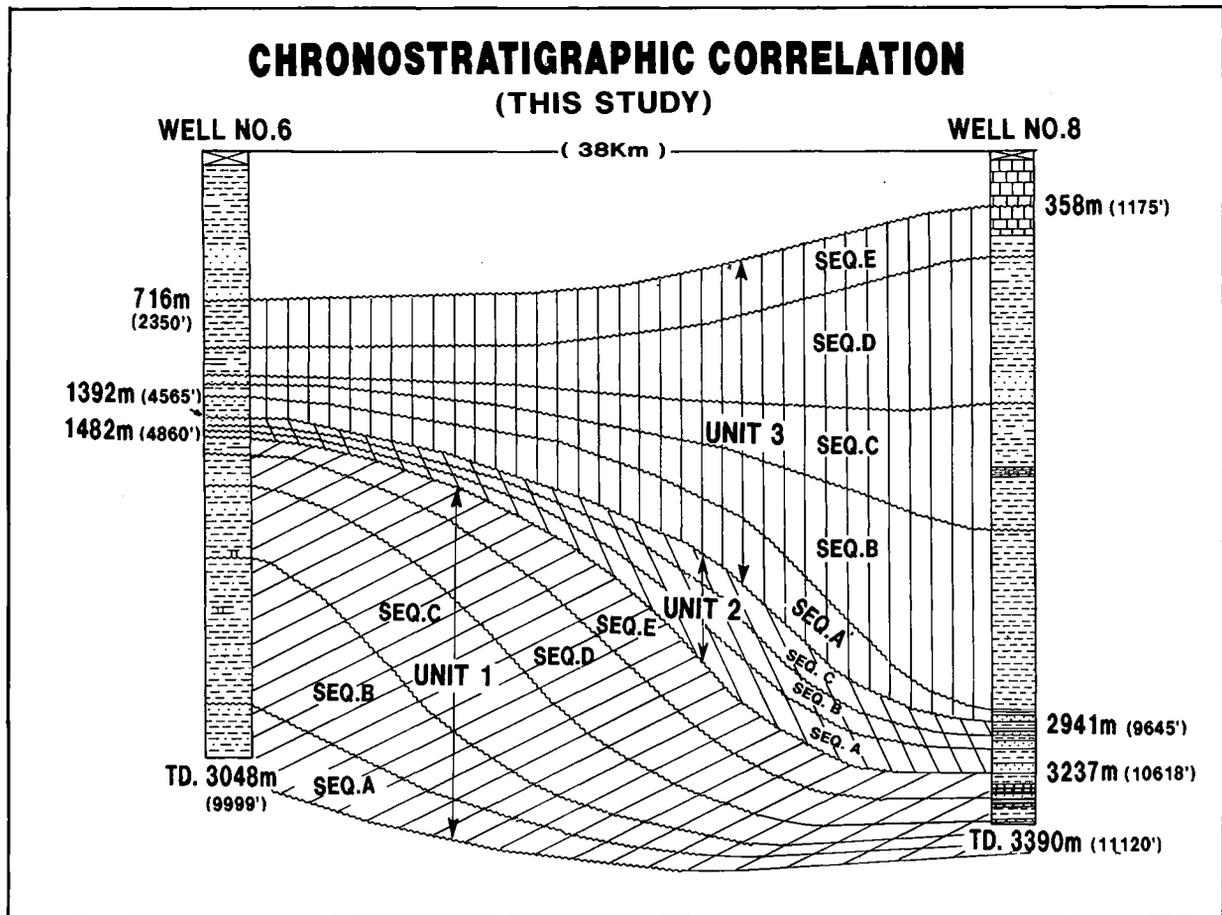
Figure 24. Chronostratigraphic correlation of well No: 6 and well No: 8.
