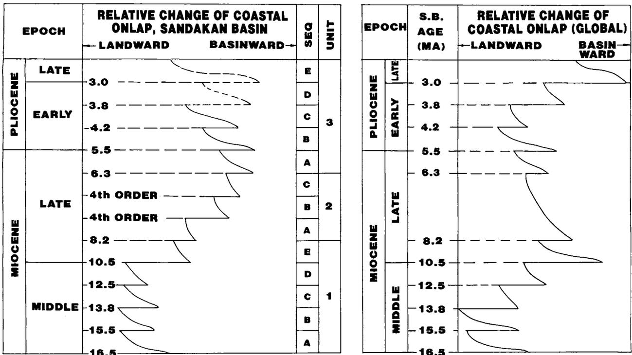
Figure 22. Comparison between coastal onlap chart of Sandakan Basin and global onlap chart of Haq *et al.* (1987).
