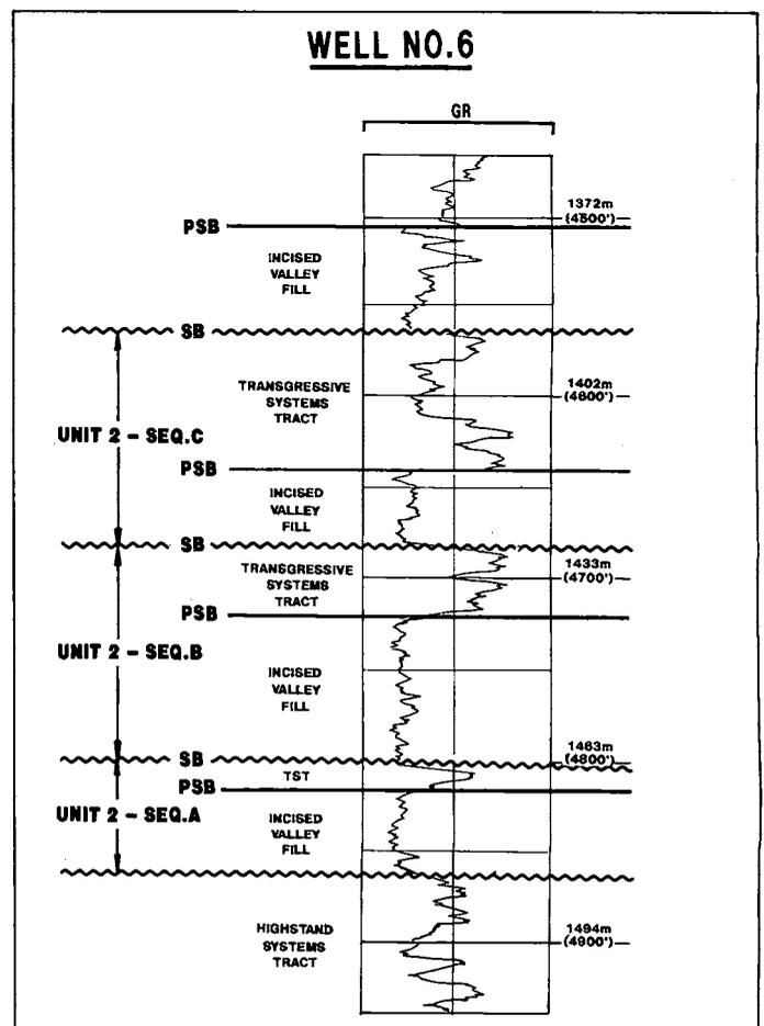
Figure 15. Interpreted system tracts in fluvial-coastal plain facies of Unit 2 at well No. 6.
