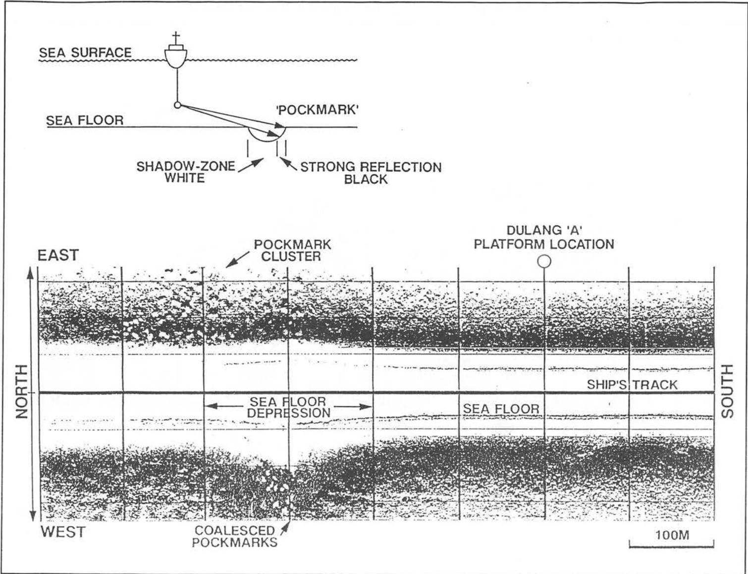
Figure 14: Sidescan sonar line E through Dulang "A" platform.
