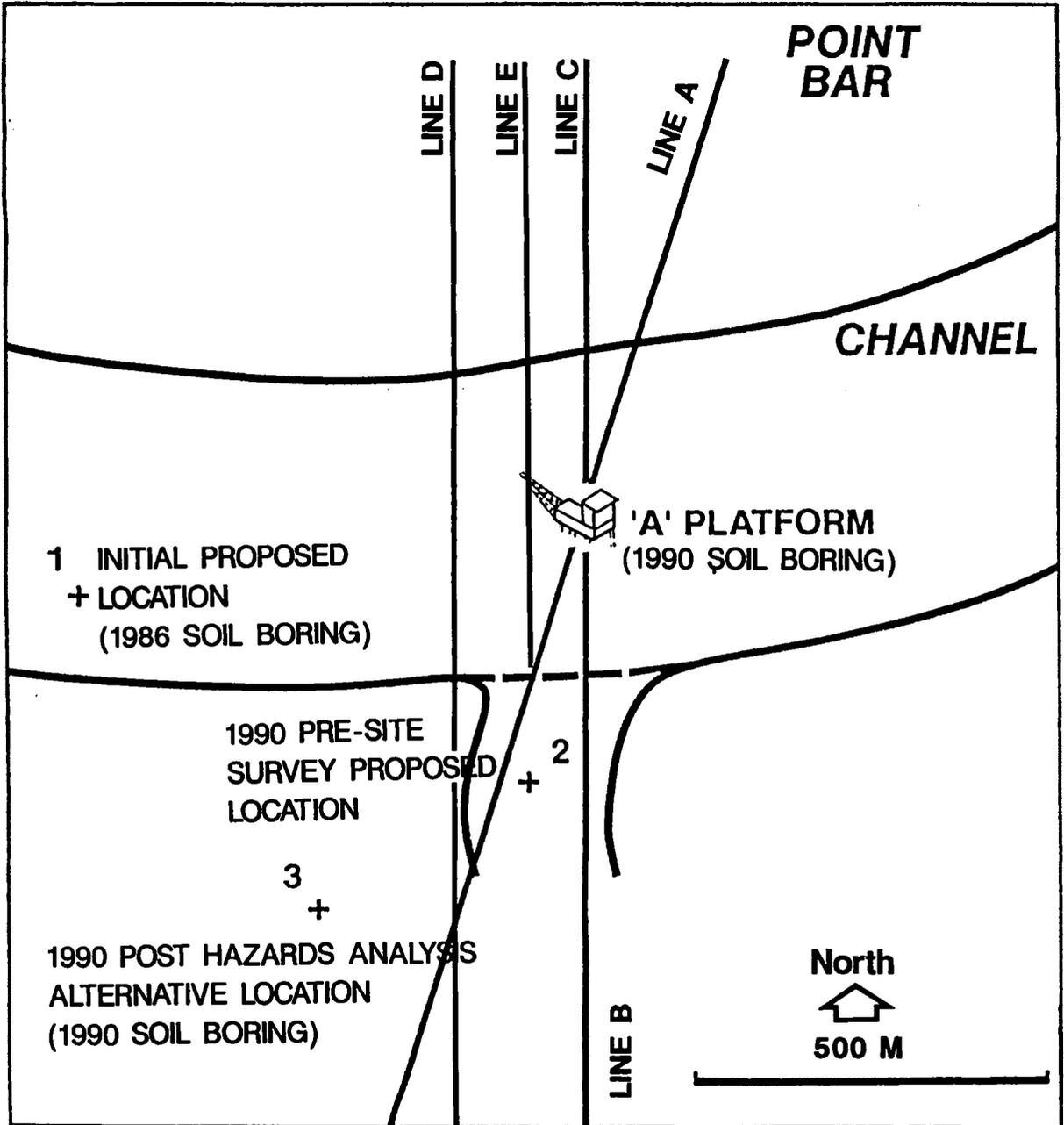
**Figure 9:** Possible locations of Dulang "A" platform with respect to channel outline interpreted from 3-D data.
