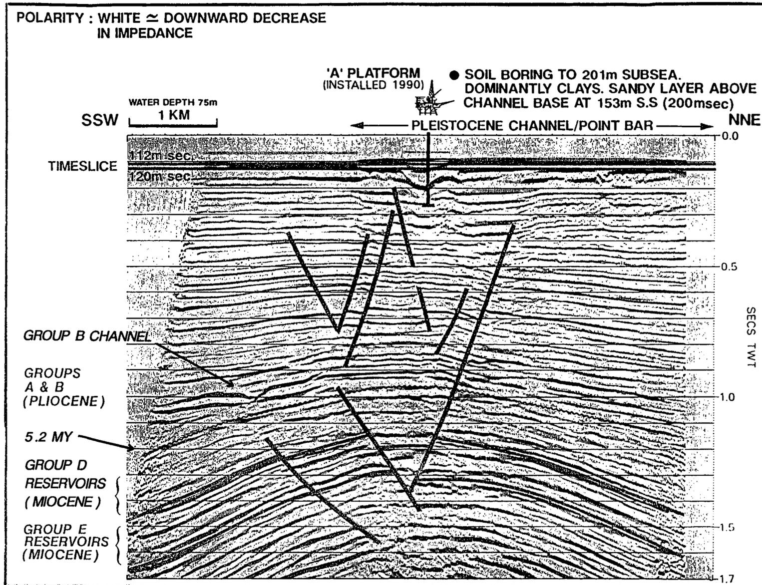
**Figure 3: 1984 3-D Line A through the "A" platform.**
