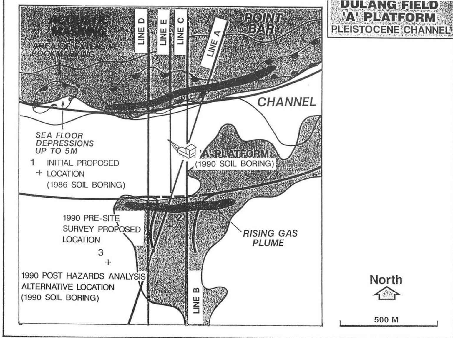
**Figure 15:** Combination of seabed and near-surface hazards mapped from 3-D seismic and site survey data.
