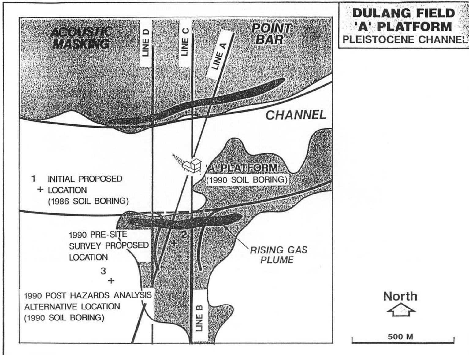
Figure 12: Area of acoustic masking and rising gas plumes interpreted from Boomer data.
