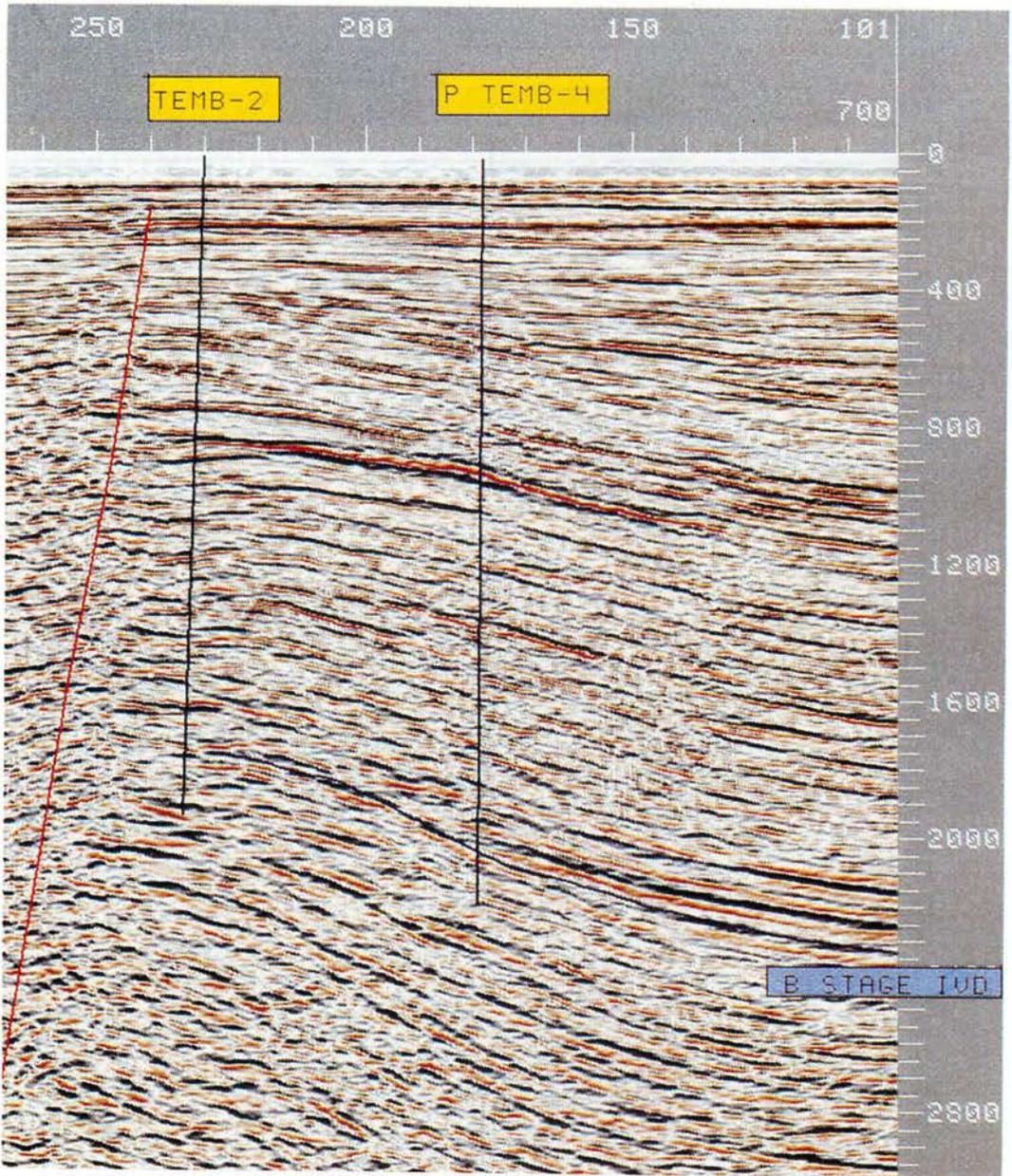
**Figure 9:** 3D seismic section showing the down lap reflector terminations of Stage IVD Sequence onto SRU in the Tembungo field.
