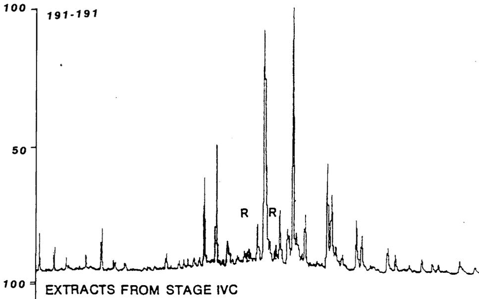
Figure 21: GCMS chromatographs of Tembungo crude and extracts from Stage IVC Sequence.
