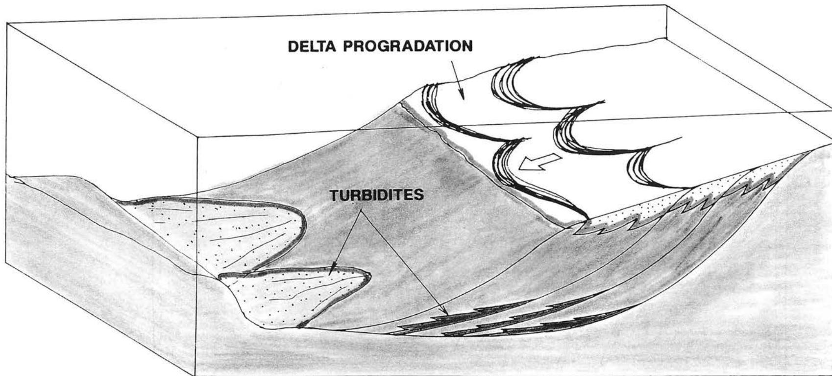
**Figure 10:** Depositional model of the Tembungo turbidite.
