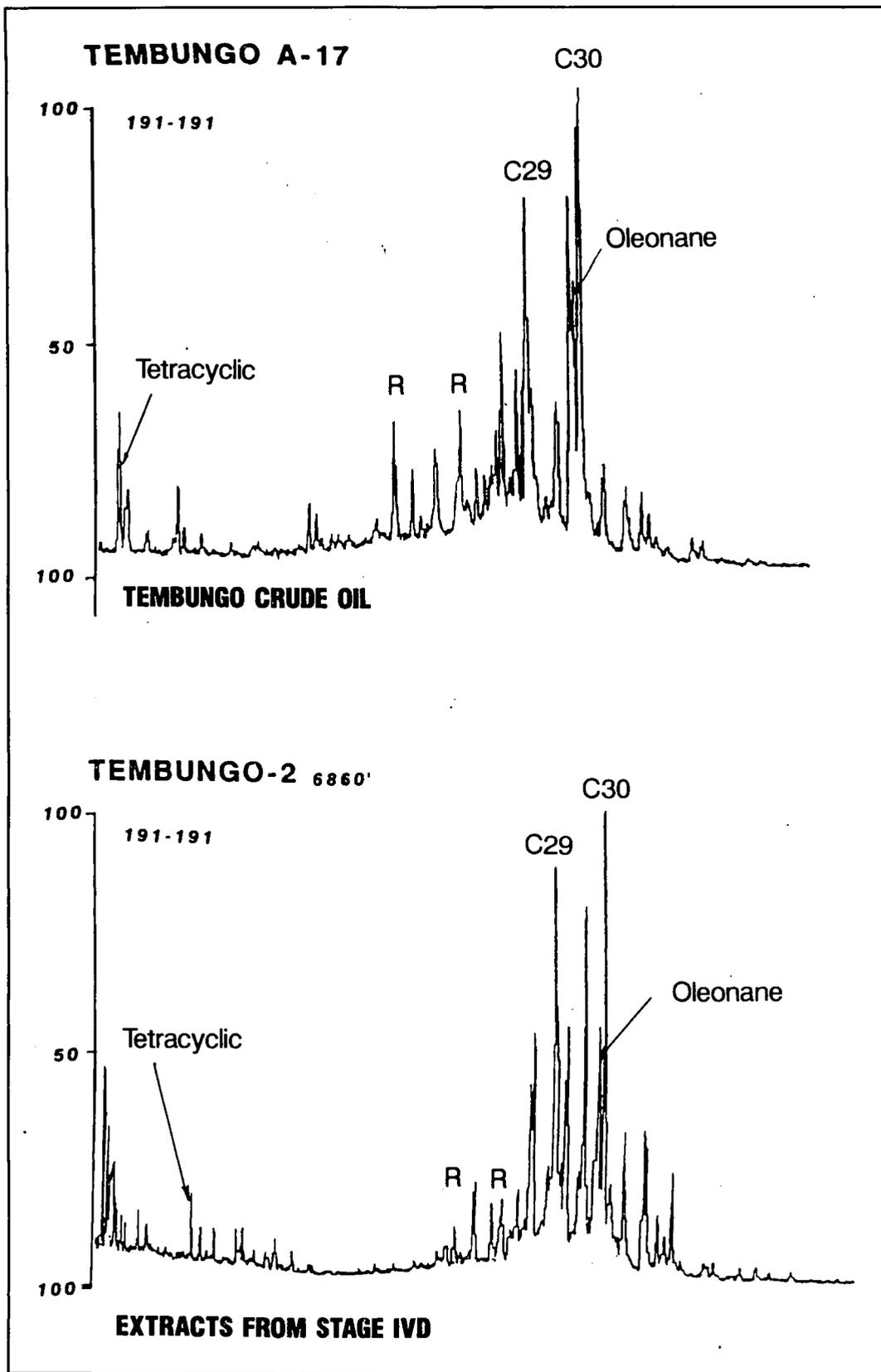
Figure 20: GCMS chromatographs of Tembungo crude and extracts from Stage IVD Sequence.
