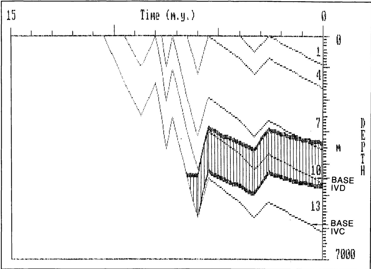
Figure 19: Maturity modelling at the northern flank of the Tembungo structure.
