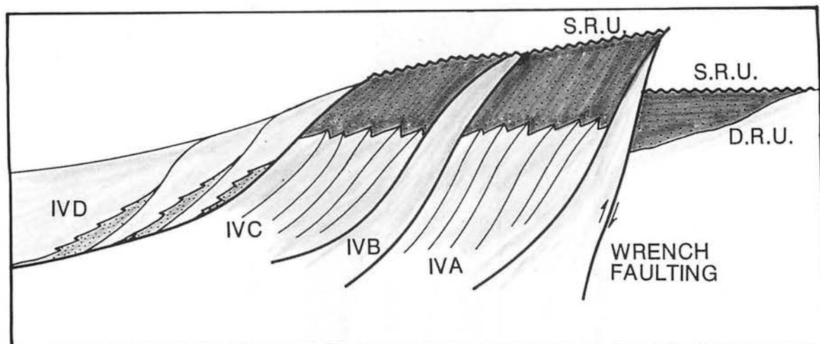
**Figure 7:** Wrench faulting post S.R.U. formation.
