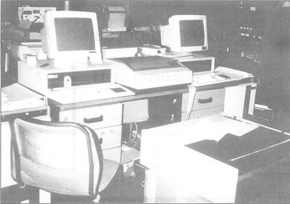
Figure 2: The shipboard processing system placed in the doghouse of the "MY" was built around two Compaq microcomputers and MicroMax (Advance Geophysical) seismic data processing software. A small Benson plotter (between the video screens) which was used mainly for velocity scans and parameter tests and a large OYO plotter (lower right) was used to produce full record sections.
