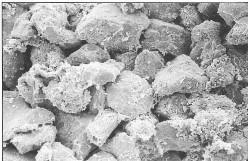
Figure 14: Scanning electron micrograph, Lower Zone— medium grained fluvial channel sandstone
