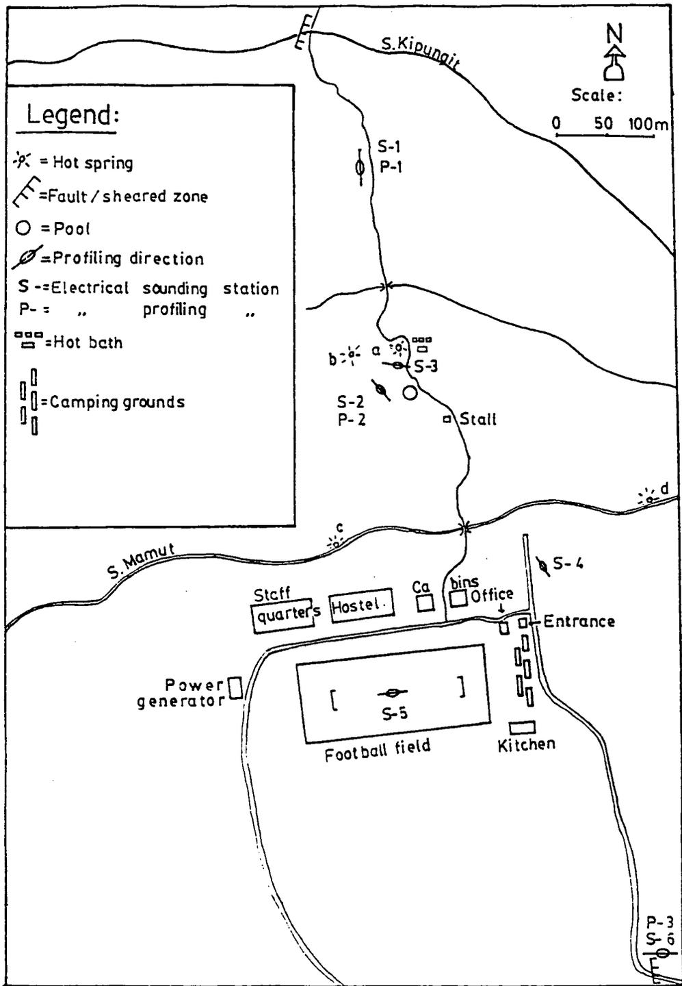
Figure 1: Location of electrical sounding and profiling stations at Poring Hot Spring.
