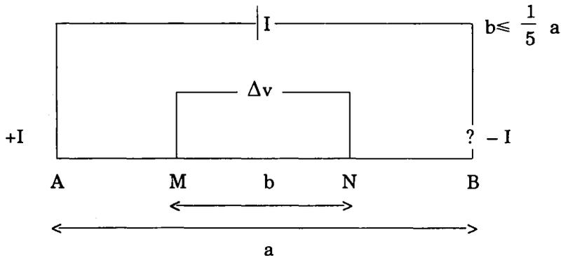
**Figure 4:** Schlumberger array used in the resistivity measurement.
