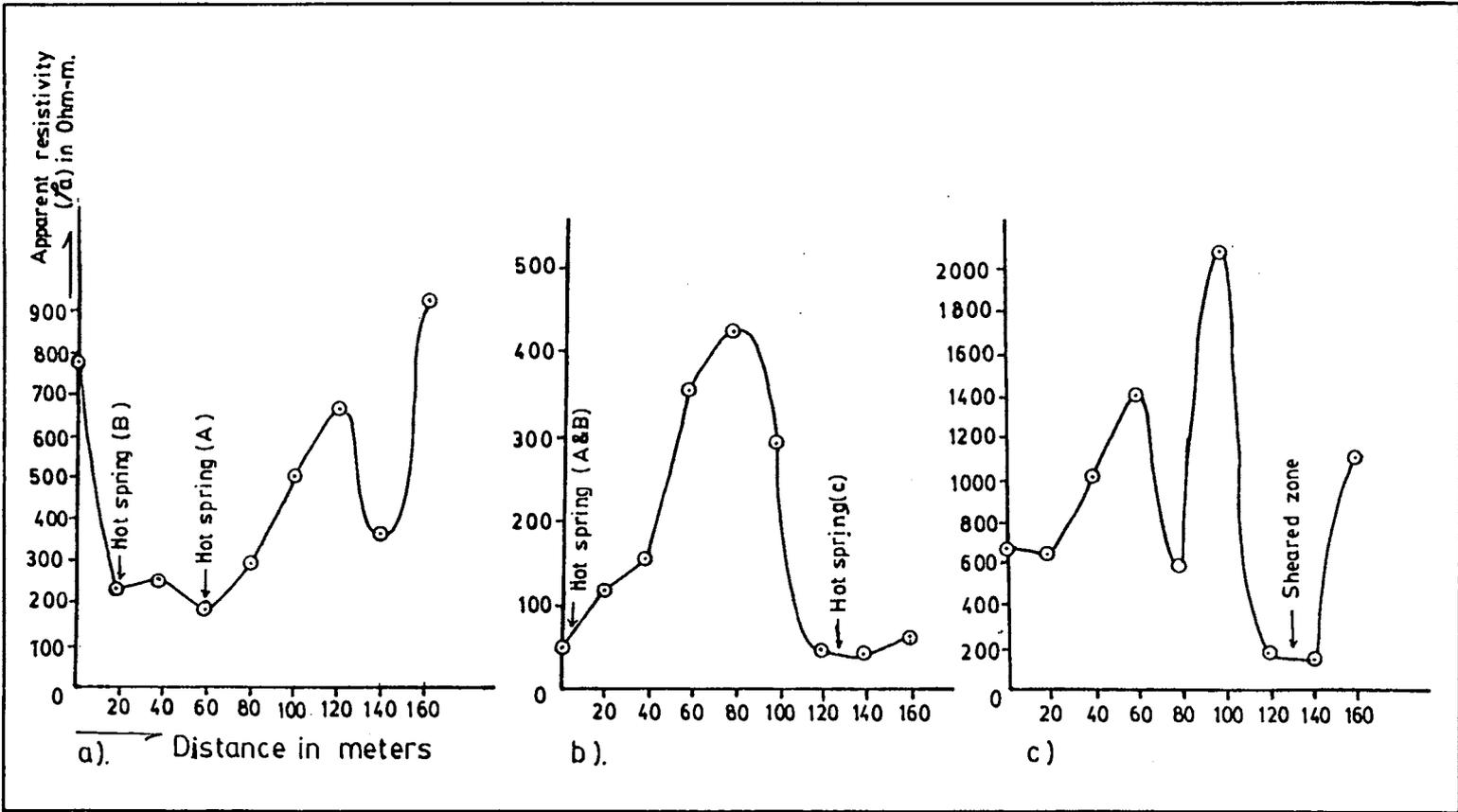
Figure 6: Resistivity profiling: a) P-1, b) P-2, and c) P-3.
