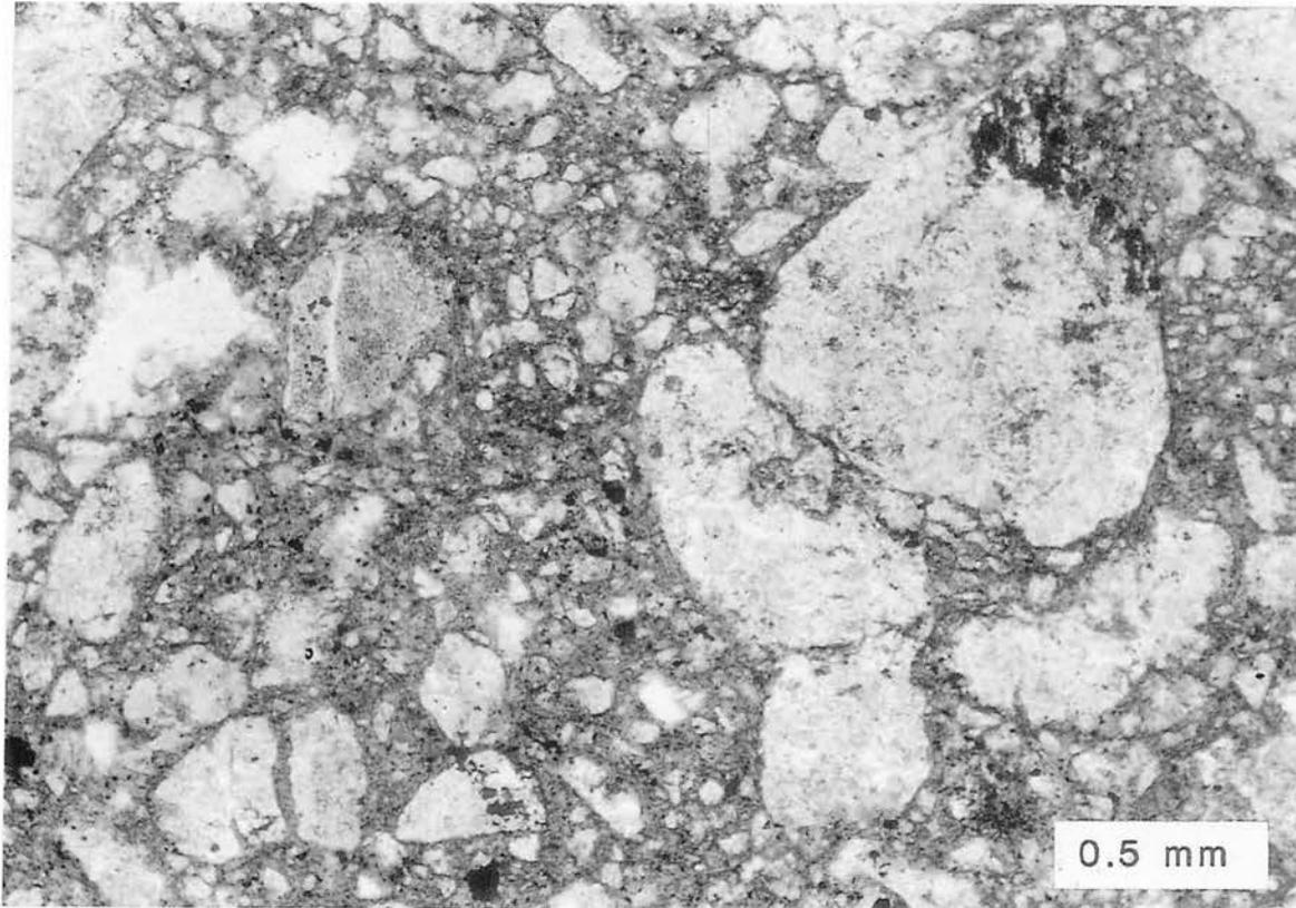
**Figure 7:** Photomicrograph from the margin of dolerite (see Figure 3D) showing fragments of rhyolitic material in a glassy groundmass, presumably formed by rapid cooling of basaltic melt, now altered to clays. 1613 m, plane-polarized light.
