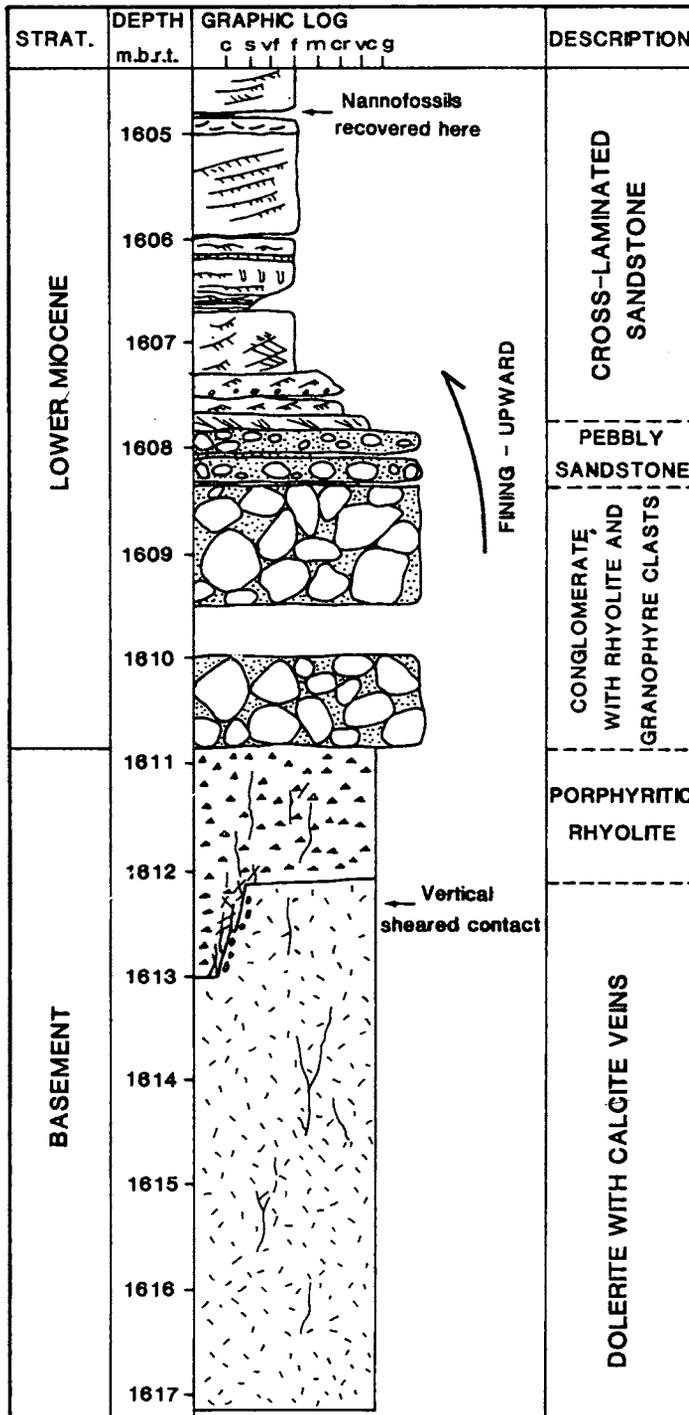
Figure 2: Summary of lithology observed in the core interval from Malong 5G-17.2 well. Core depth in meters below rotary table (m.b.r.t.).
