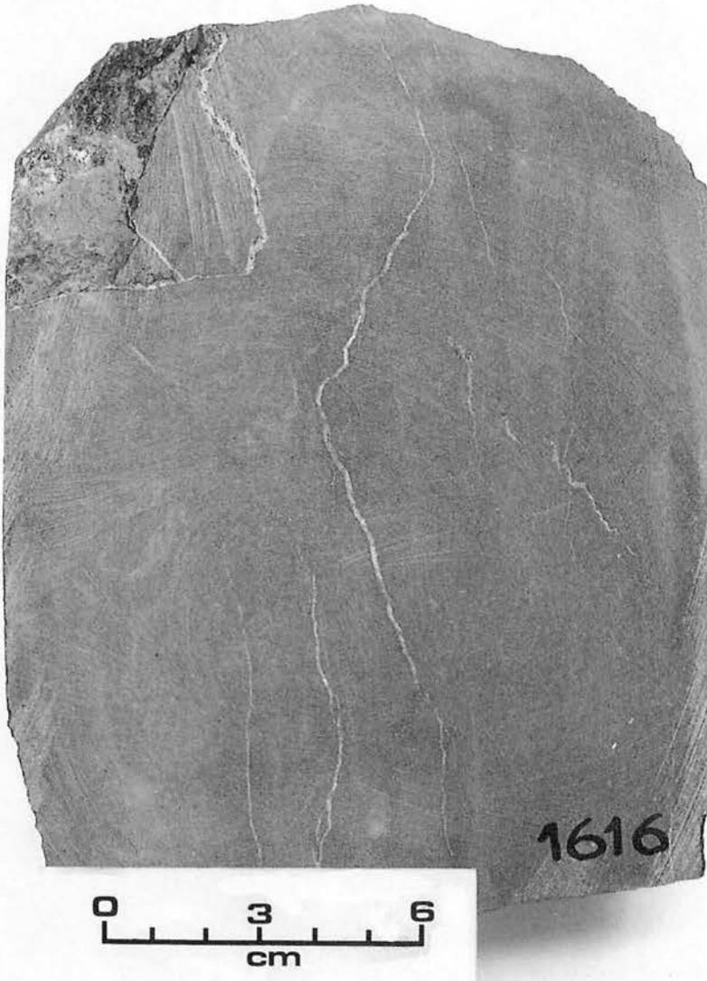
**Figure 5:** Core sample of dolerite showing fine-grained texture and thin calcite-filled fractures. Depth: 1616 m.
