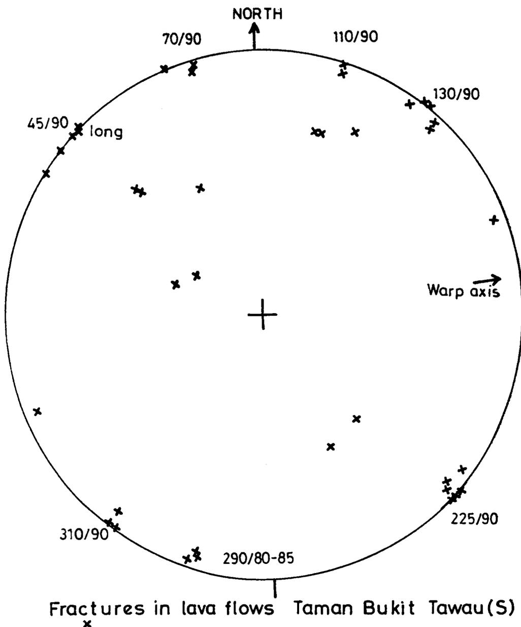
**Figure 5:** Lower hemisphere, equal-area plot of fractures in lava flows at the entrance to Taman Bukit Tawau (see Figure 4). The warp axis is exposed in the valley wall at the fall. The low-angle fractures may represent flow planes. The SE-SW vertical fractures form a prominent set.
