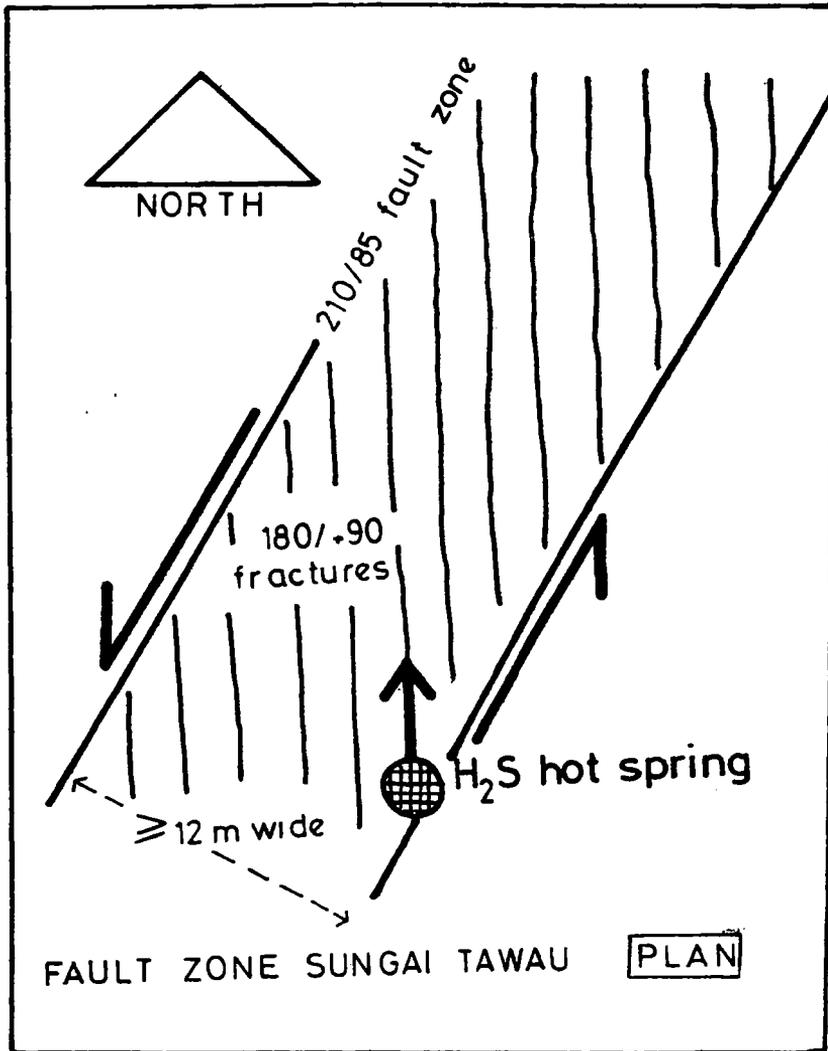
**Figure 3:** A wide transcurrent fault zone through ?Pliocene lava at the hot spring on Sungai Tawau, some 3 km north from the Park's entrance.
