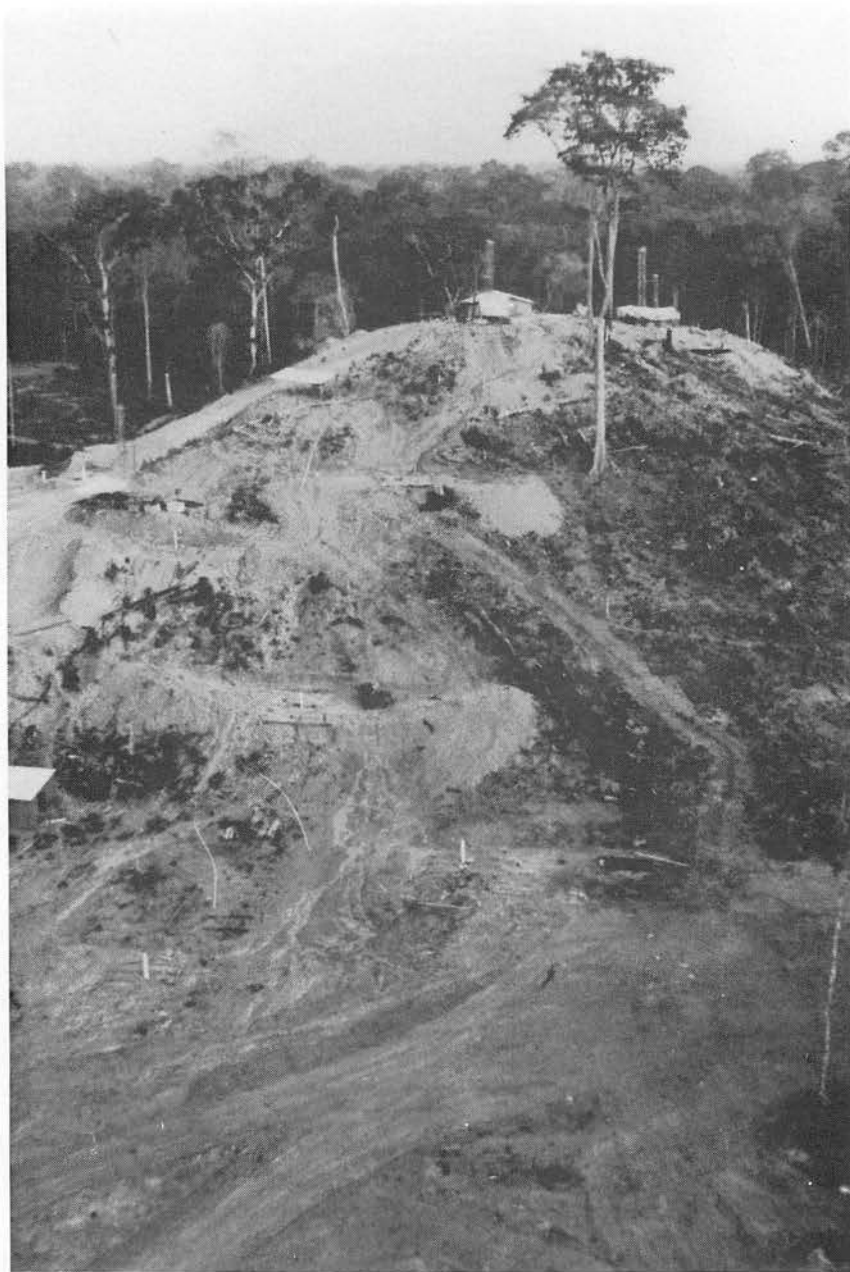
Figure 5A: A photograph of tin-rich hill known as Morro Potosi in the tin-field of Rondonia, Brazil. In recent years this hill has been completely eliminated during the recovery of the cassiterite that it contained. The hill was a strange feature in the Rondonian environment and it occurred at the hub of the tin-bearing areas.
