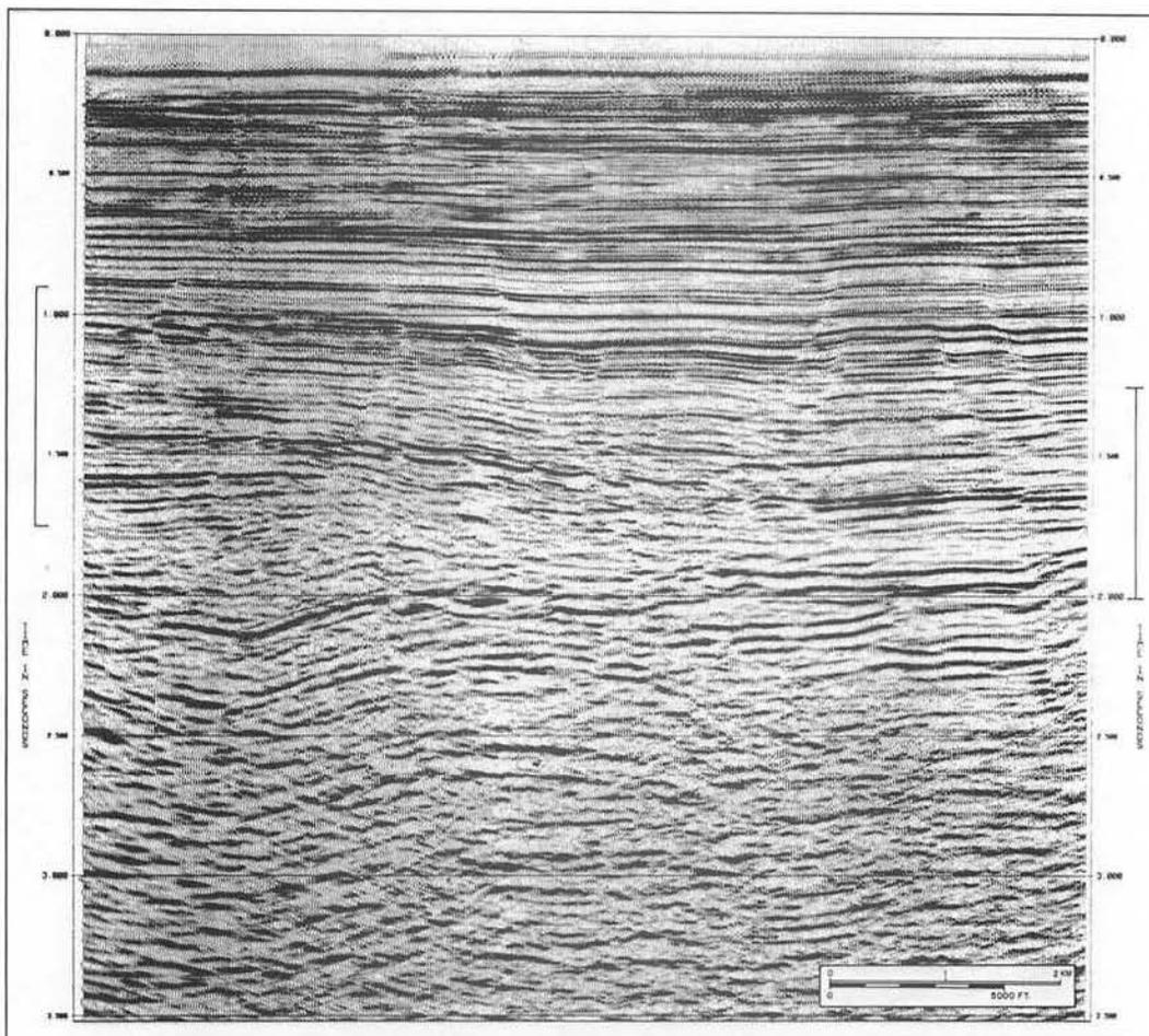
Figure 3: Seismic line obtained from a 3D seismic survey along the same subsurface trajectory as the 2D line (Fig. 2) after binning to correct for feathering but with 2D inline migration only.
