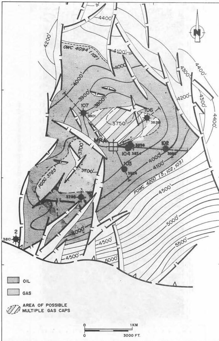
Figure 9: DEVELOPMENT AREA MP-A. Depth contour map at reservoir level based on 3D seismic including the drilling results.
