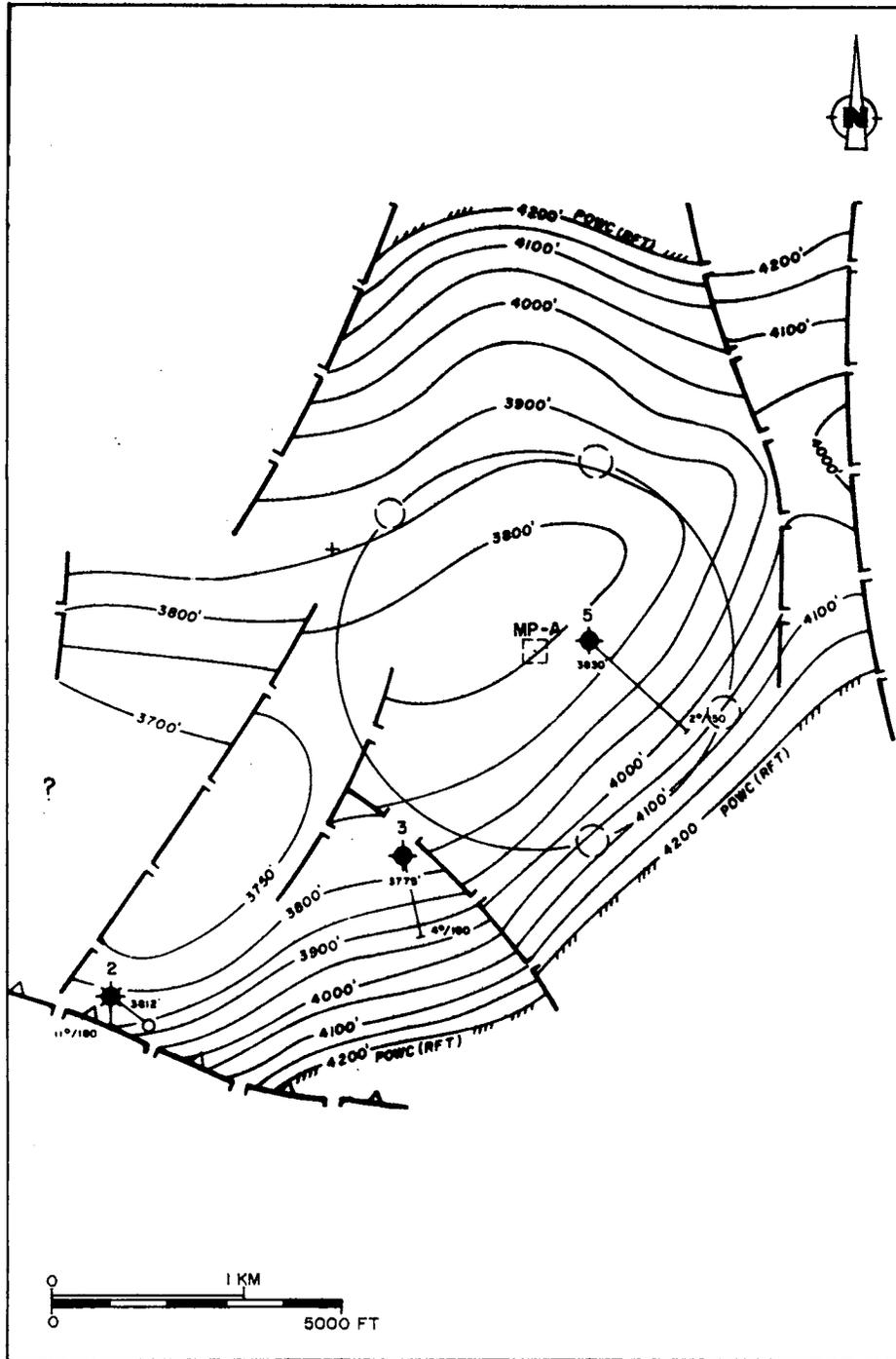
Figure 7: DEVELOPMENT AREA MP-A. Depth contour map at reservoir level based on 2D seismic data.
