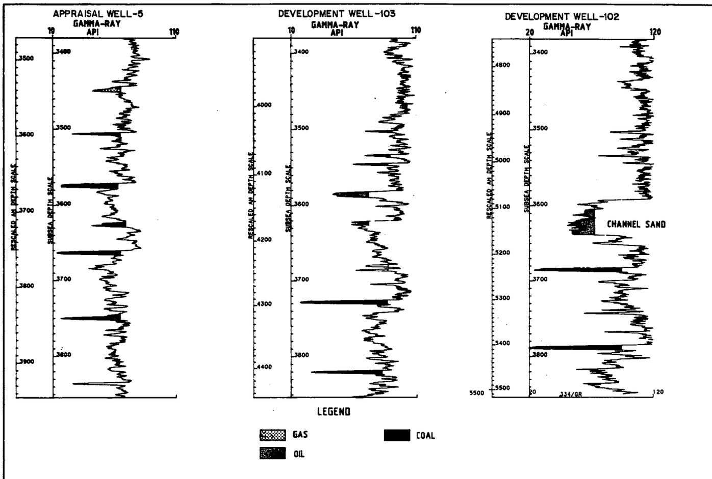
Figure 14: DEVELOPMENT AREA MP-A. Gamma ray logs from wells -5, 103 and -102.
