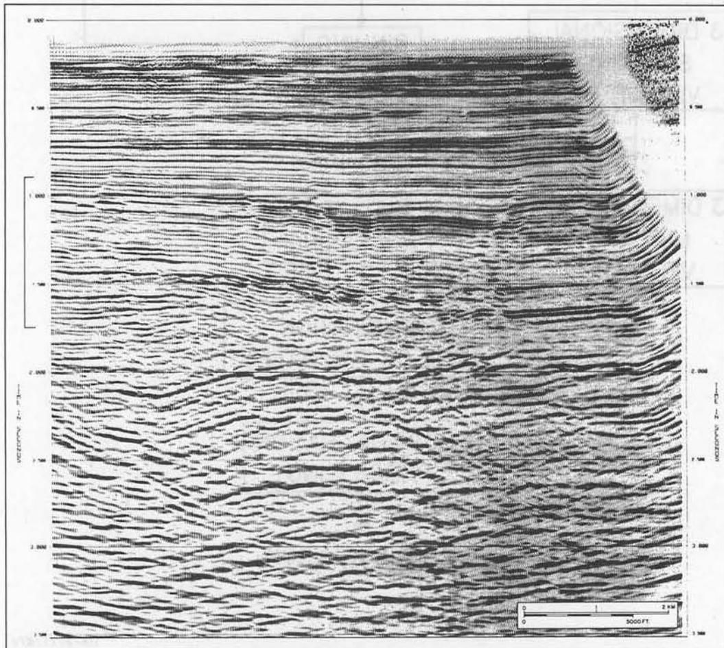
Figure 2: Seismic line obtained from a 3D seismic survey processed as a conventional 2D line (no binning and 2D migration only).
