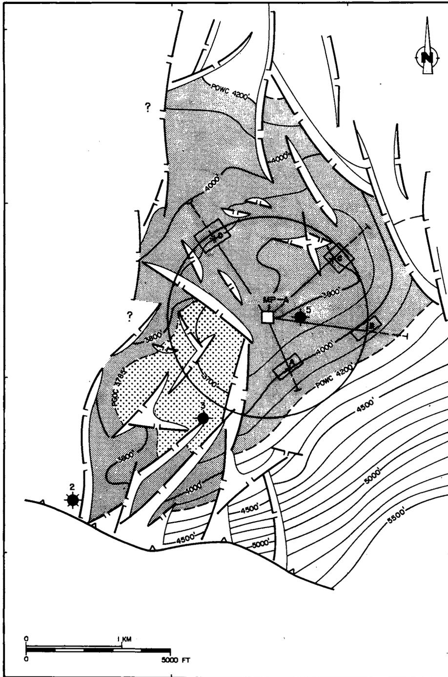
Figure 8: DEVELOPMENT AREA MP-A. Depth contour map at reservoir level based on 3D seismic data.
