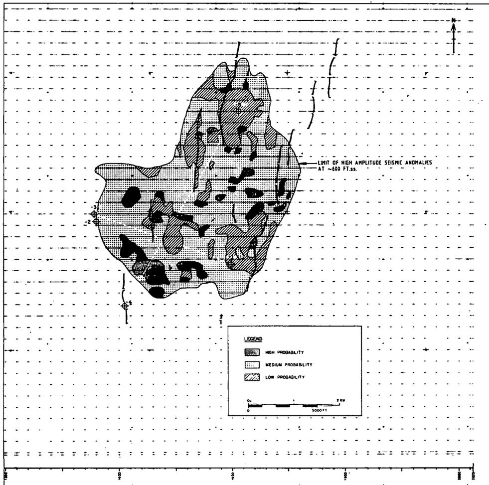
Figure 11: Map of potential drilling hazards based on time-slice interpretation.
