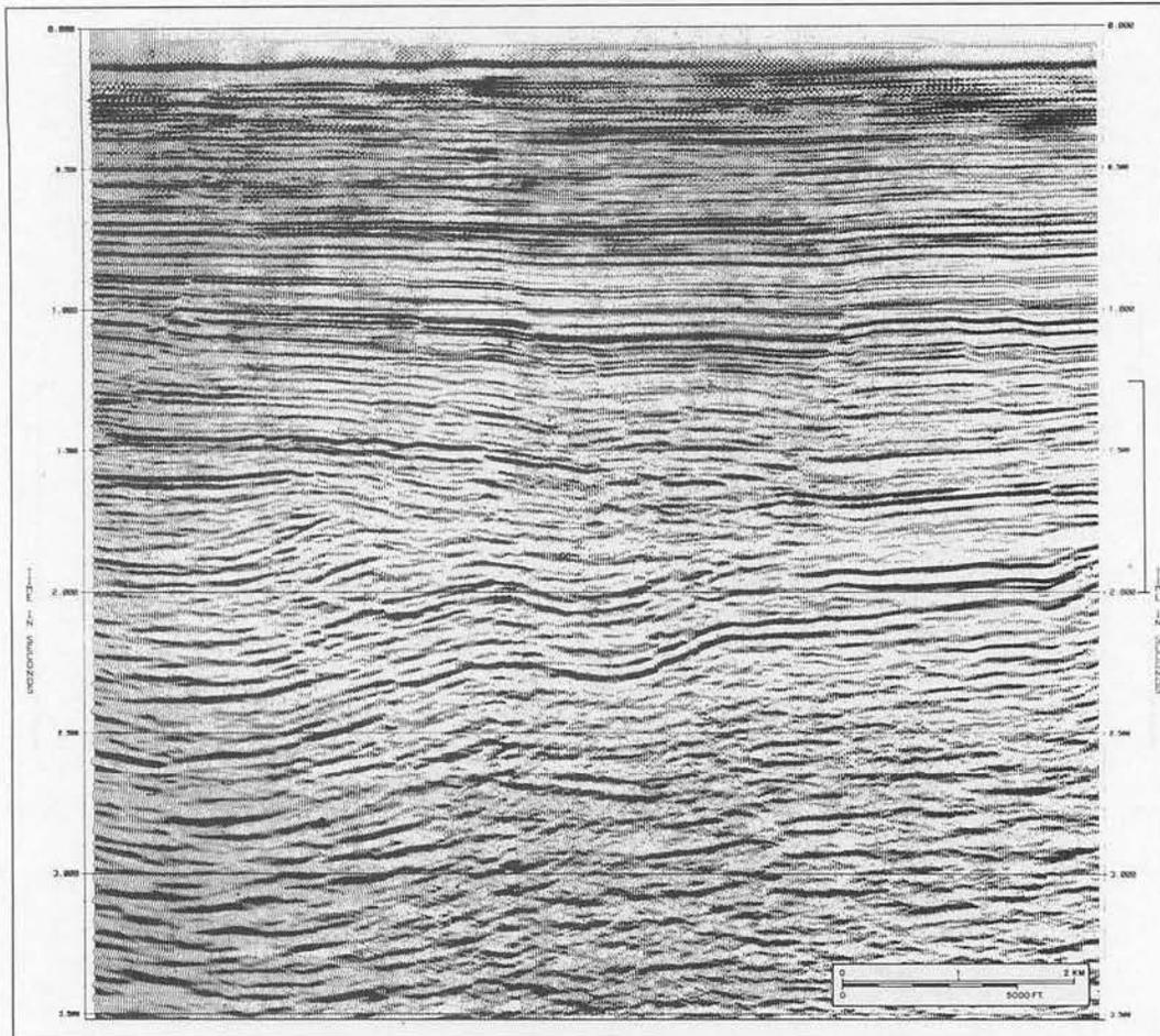
Figure 4: Same seismic line as shown in figure 3, but after 3D migration.
