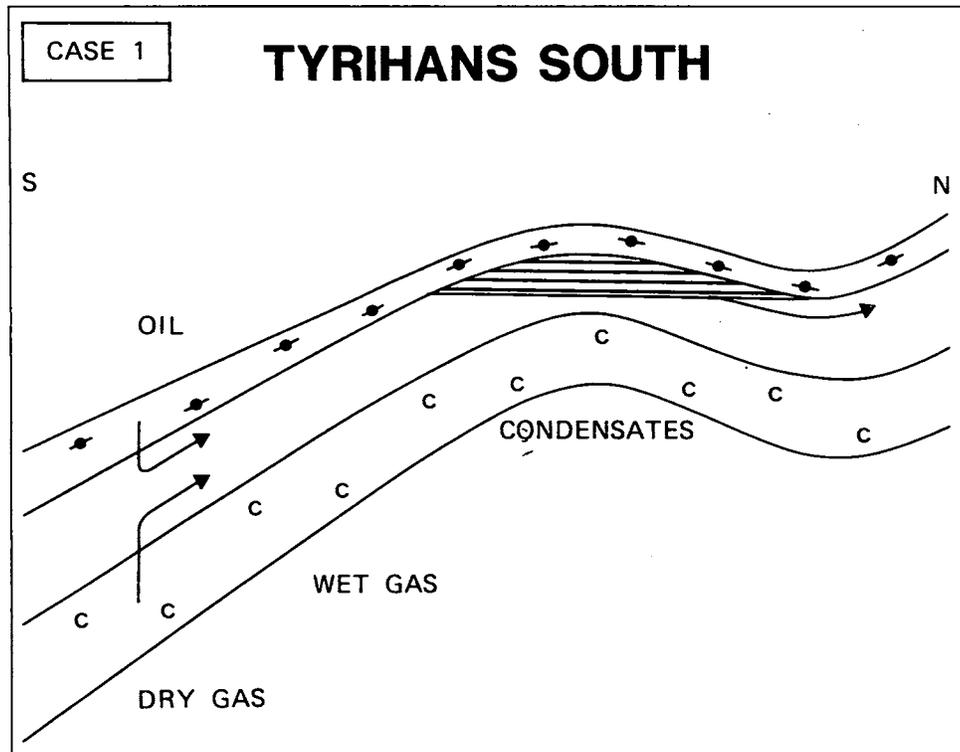
Figure 15: Case 1. Sketch of hydrocarbon migration and trapping conditions at Tyrihans South.
