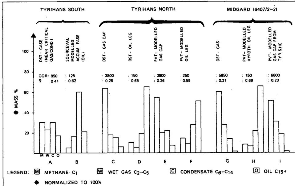
Figure 13: Comparison between measured and modelled hydrocarbon compositions at Tyrihans and Midgard fields.
