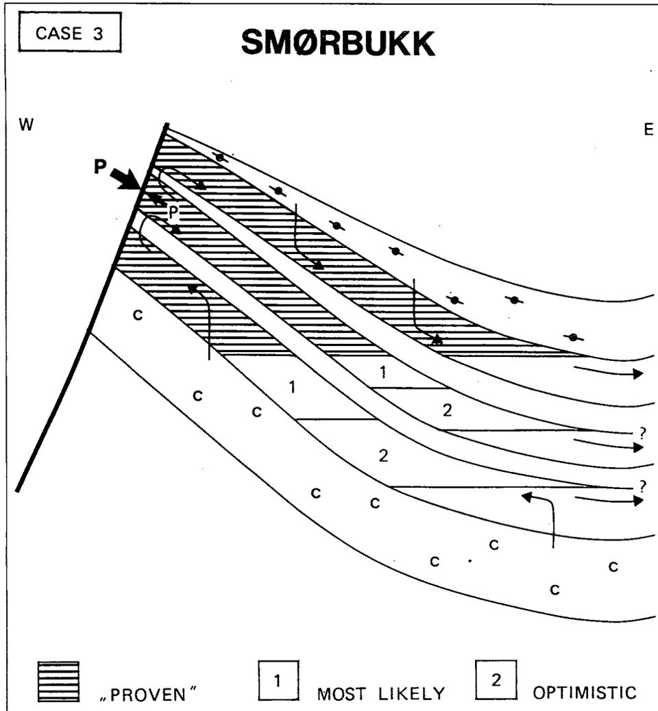
Figure 17: Case 3. Sketch of hydrocarbon migration trapping conditions at Smørbukk
