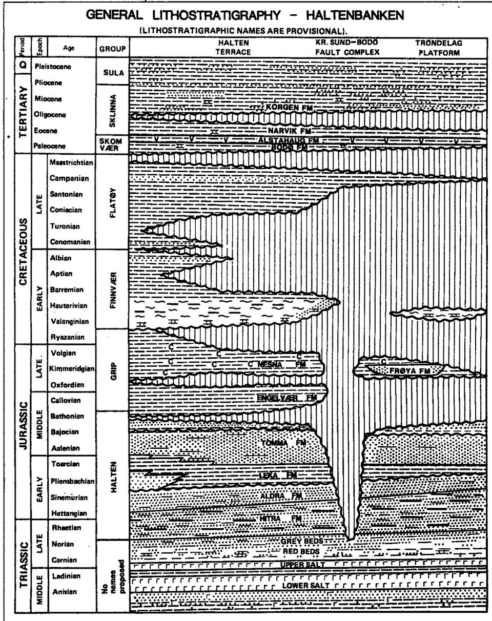
Figure 4: Lithostratigraphic units at Haltenbanken. Generalized east-west section.
