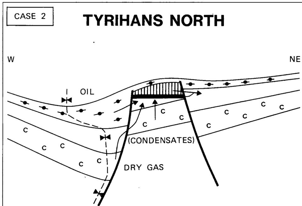
Figure 16: Case 2. Sketch of hydrocarbon migration and trapping conditions at Tyrihans North.
