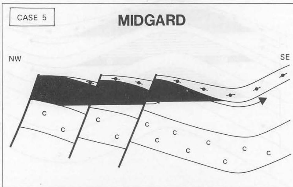
Figure 19: Case 5. Sketch of hydrocarbon migration and trapping conditions at Midgard.
