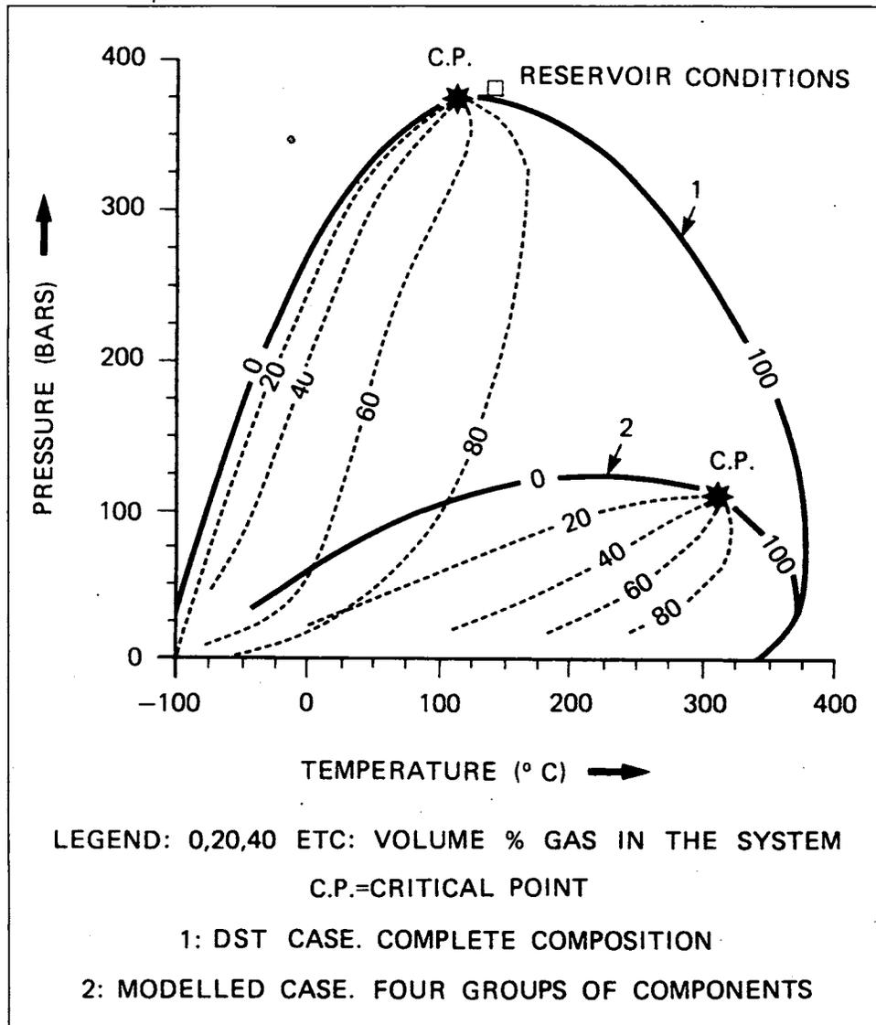
Figure 12: Comparison between measured and modelled phase envelopes at Tyrihans South.
