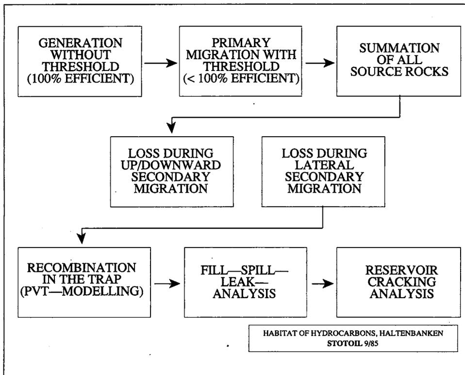
Figure 5: Generalized flow chart of the computer programme SOURCEVAL.
