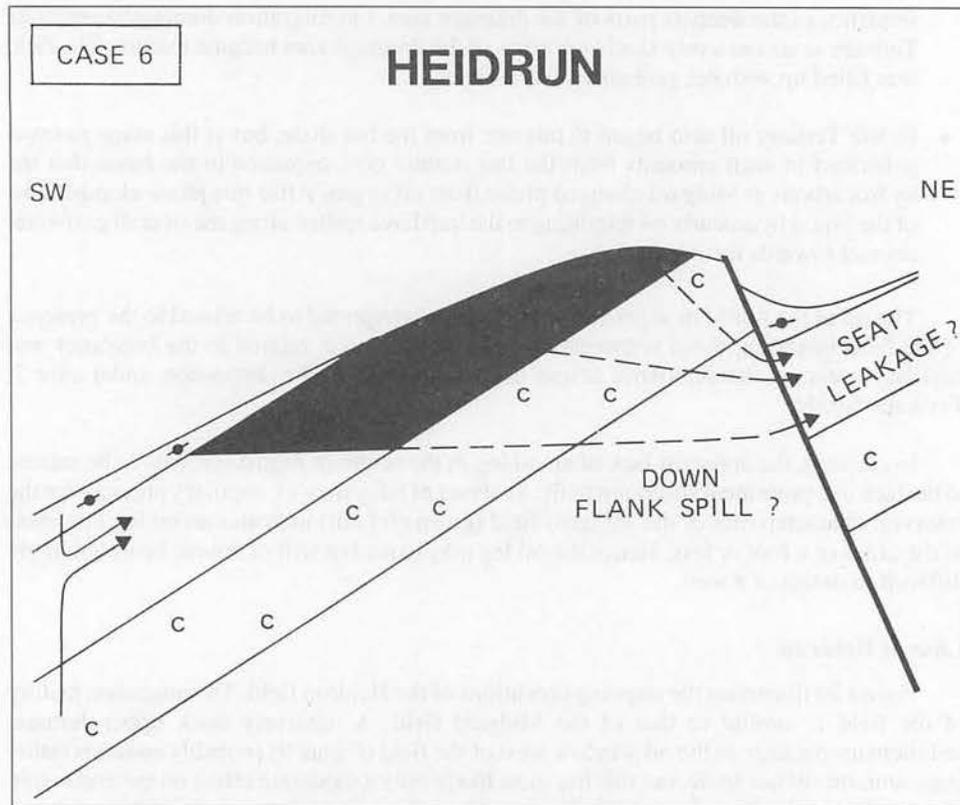
Figure 20: Case 6. Sketch of hydrocarbon migration and trapping conditions at Heidrun.
