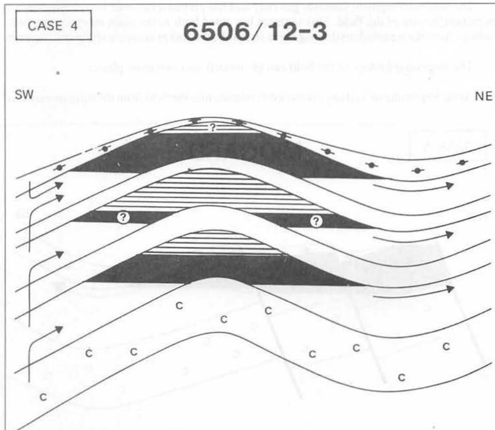
**Figure 18:** Case 4. Sketch of hydrocarbon migration and trapping conditions at 6506/12-3 ( Smørbukk satellite).
