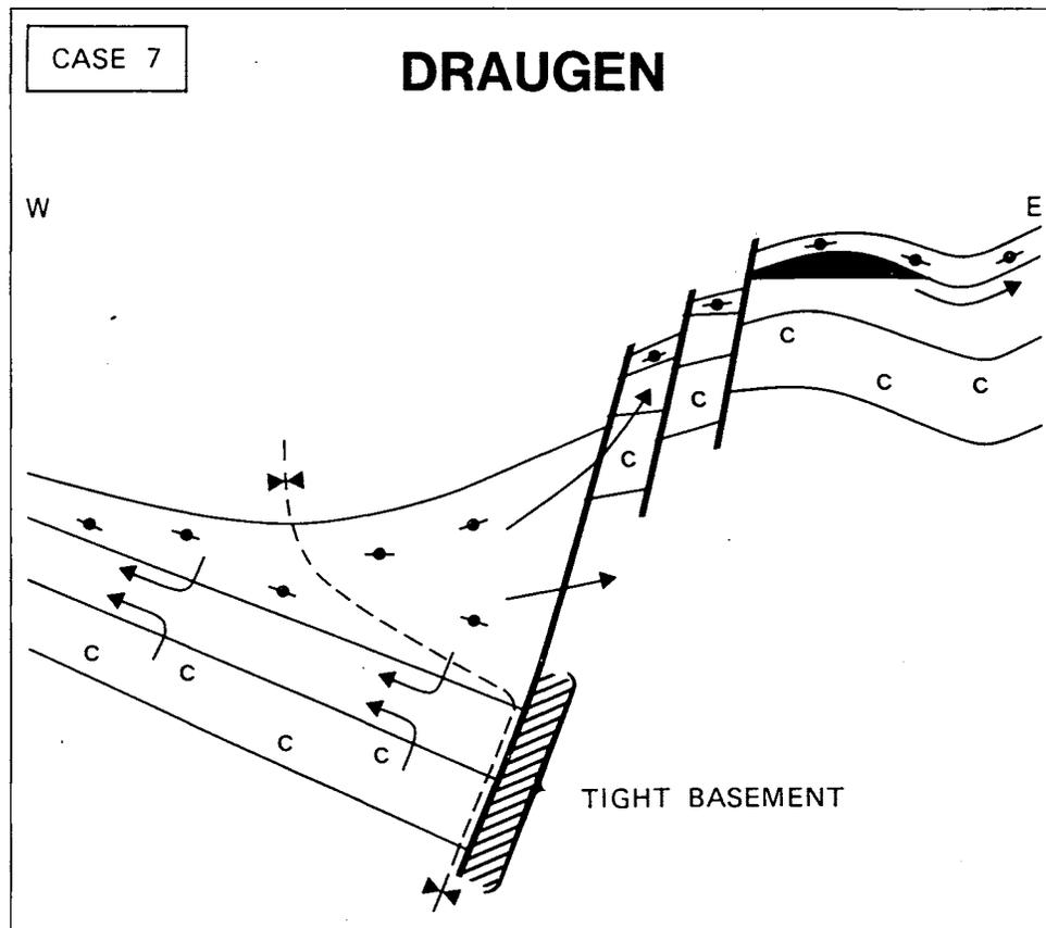
Figure 21: Case 7. Sketch of hydrocarbon migration and trapping conditions at Draugen.
