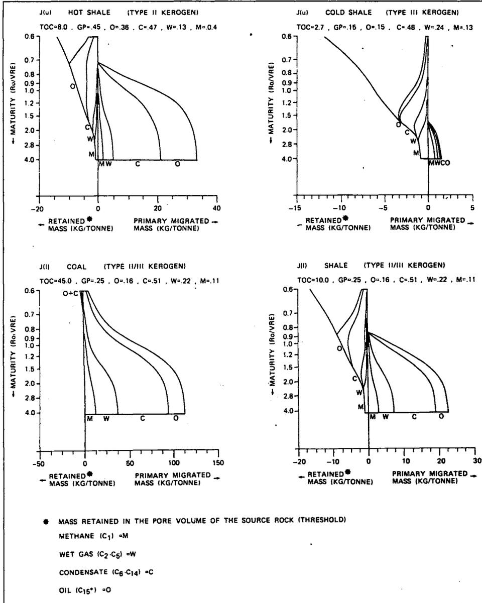
Figure 6: SOURCEVAL diagrams for representative source rocks at Haltenbanken.
