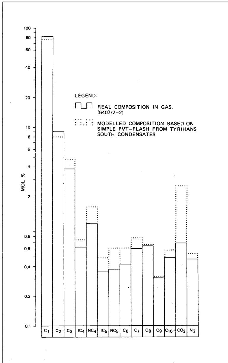
Figure 14: Detailed comparison between measured and modelled hydrocarbon composition at Midgard.
