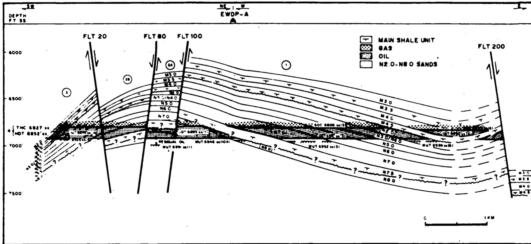
Fig. 2. Erb West Top M4.0 Map and Geological Cross-section of M3.0 - N8.0 reservoir
