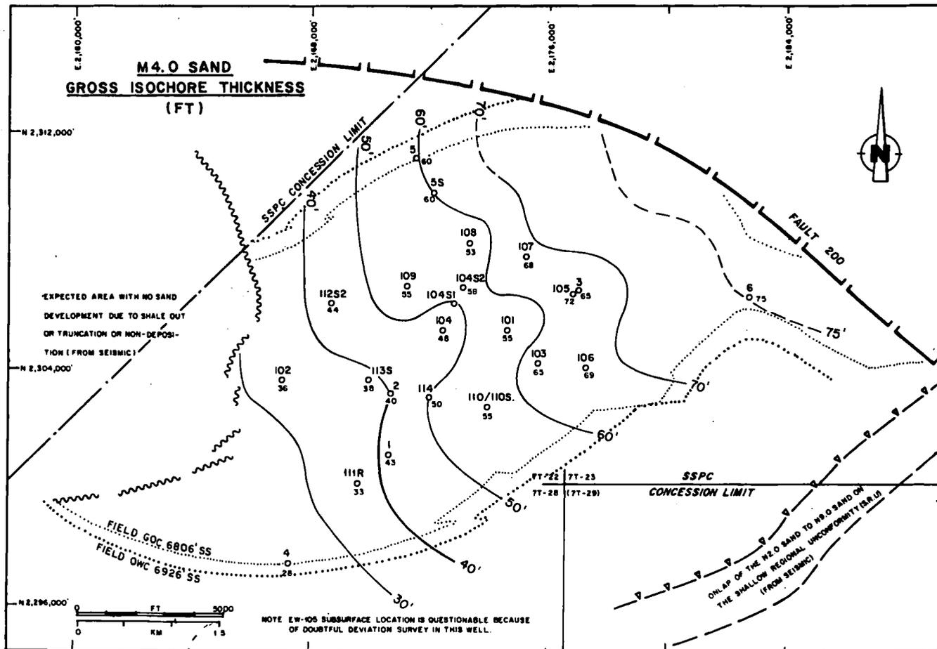
Fig. 23. M4.0 Sand Gross Isochore Thickness
