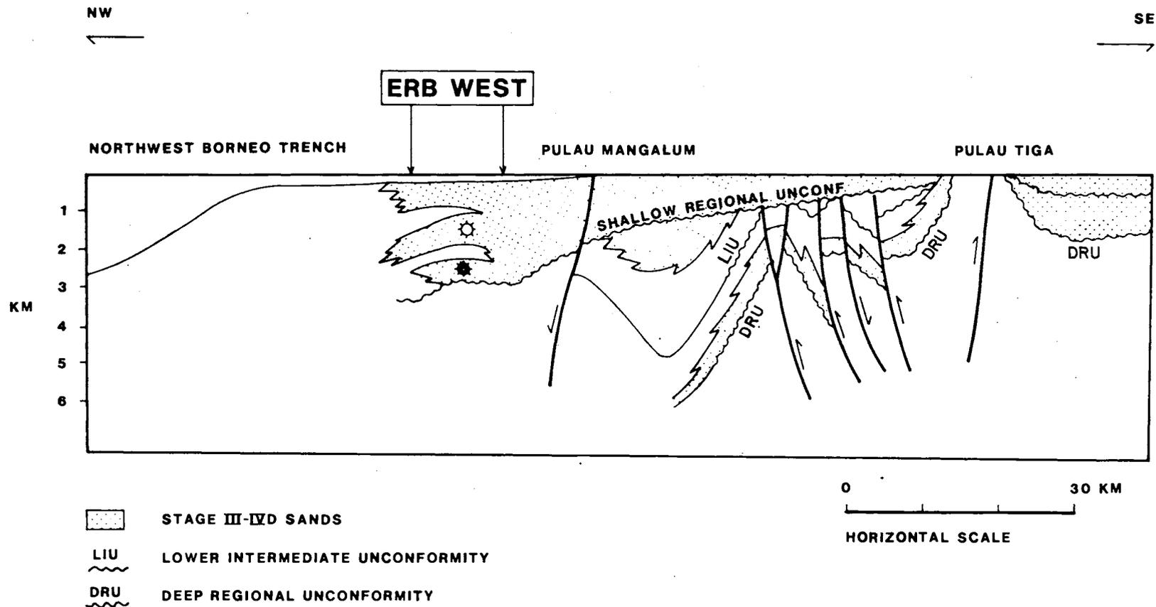
Fig. 6. Regional Geological Cross-section through West Sabah Offshore
