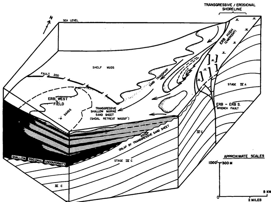
Fig. 13. Erb West Depositional Model for Stage IVD Sand Reservoirs
