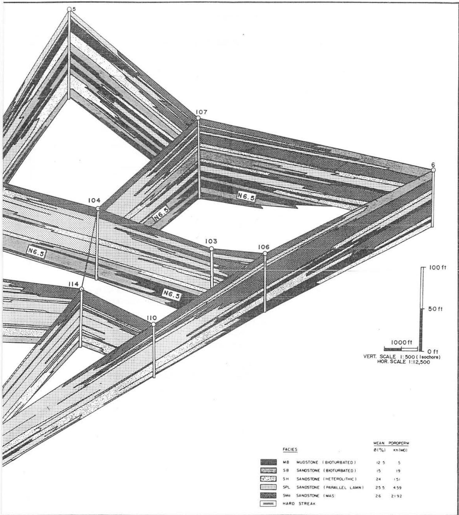
Fig. 21. Fence Diagram of Facies Distribution for the N6.0 reservoir sands
