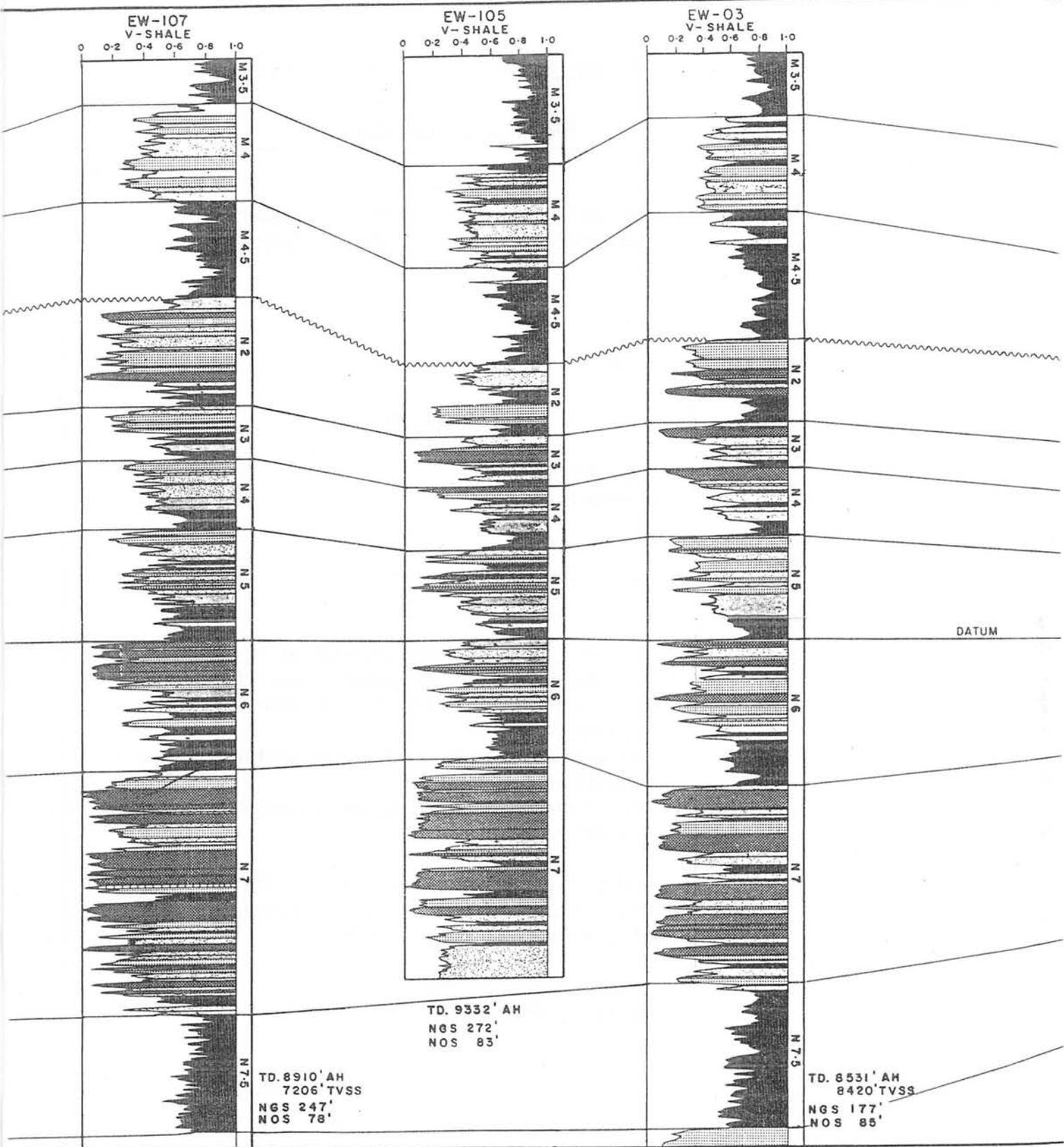
Fig. 17. Correlation Panel of M4.0 - N8.0 reservoirs
