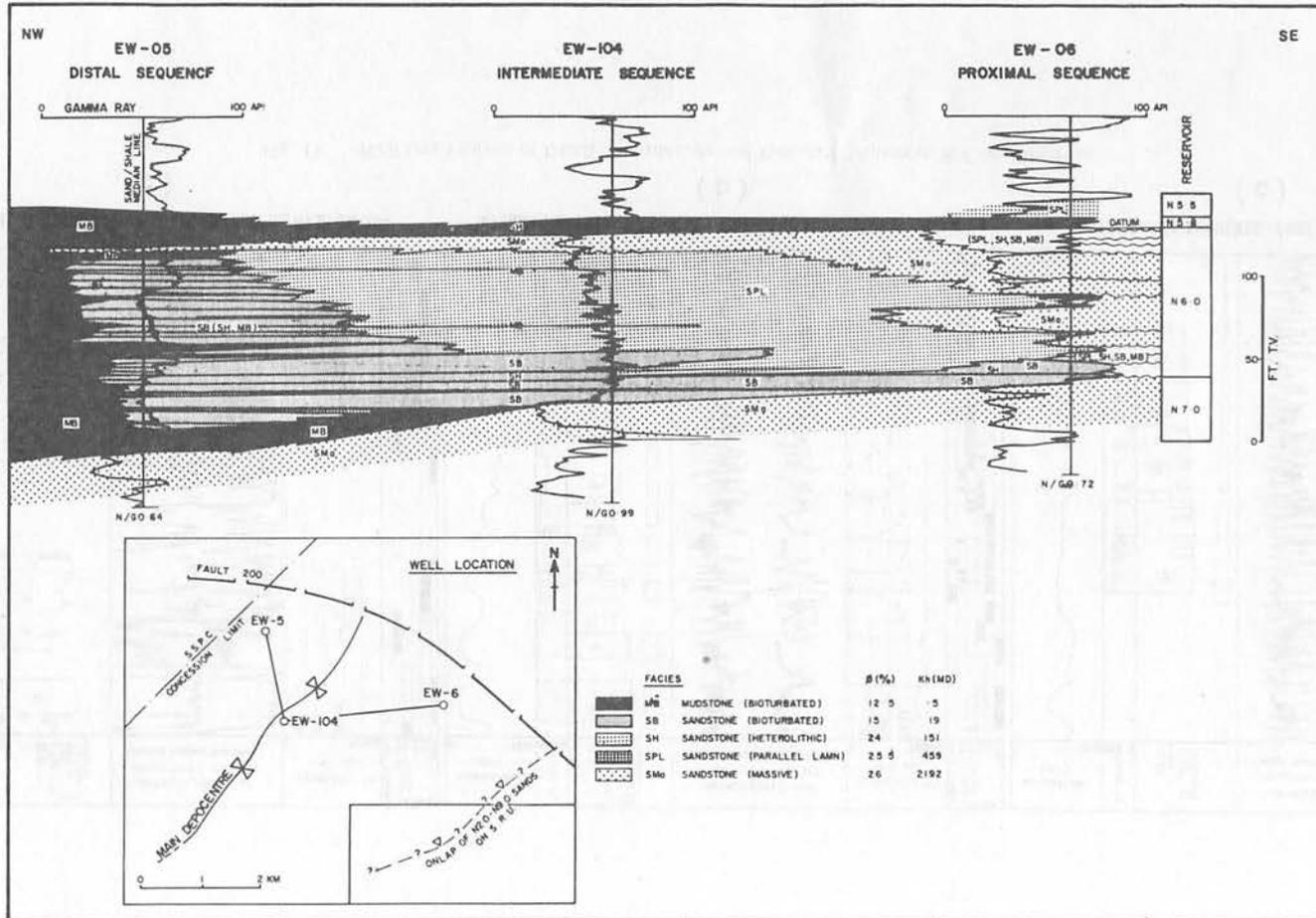
Fig. 10. Well Log Profiles and Facies Distribution for N6.0 Sand
