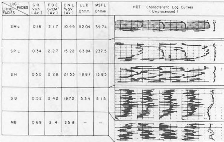
LOG-FACIES CUT-OFF IN OIL BEARING INTERVALS OF M & N RESERVOIRS (BASED ON EW-4.5 & 104)
