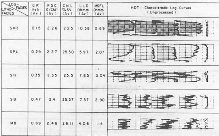
LOG-FACIES CUT-OFF IN WATER BEARING INTERVALS OF M & N RESERVOIRS (BASED ON EW-4 & 5)
