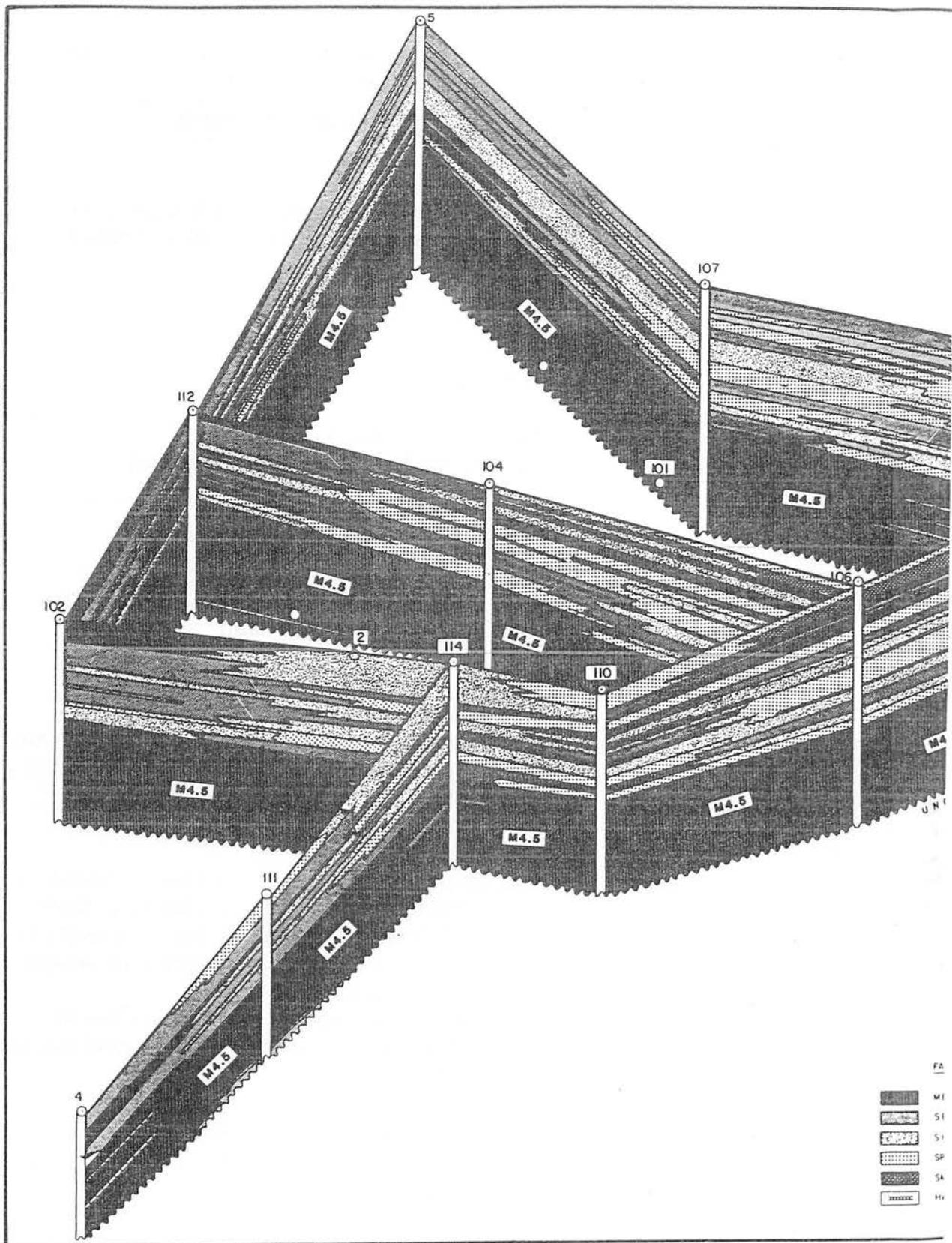
Fig. 25. Fence Diagram of Facie, Distribution for the M4.0/M4.5 reservoir sands and
