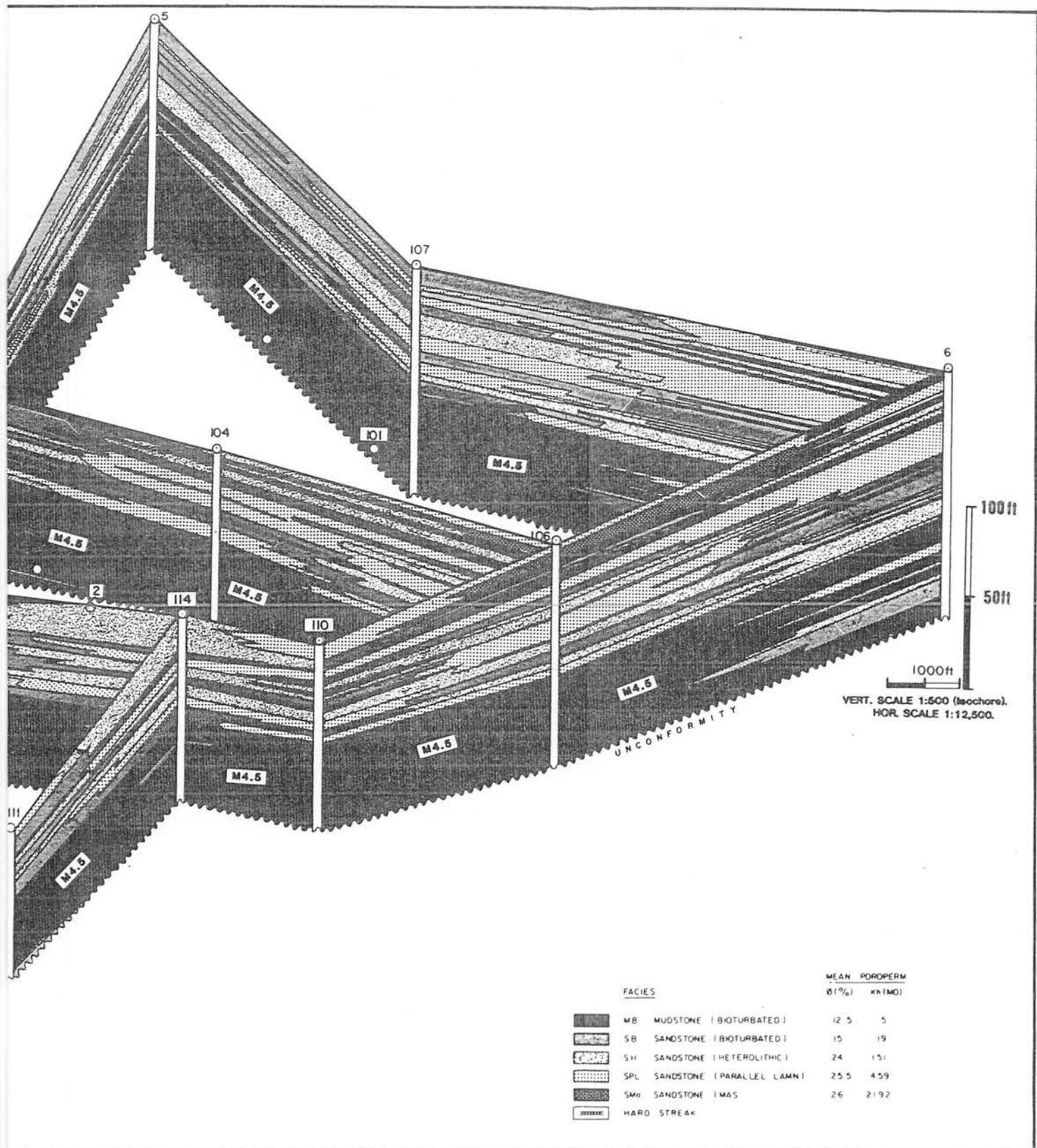
Fig. 25. Fence Diagram of Facie, Distribution for the M4.0/M4.5 reservoir sands and shales
