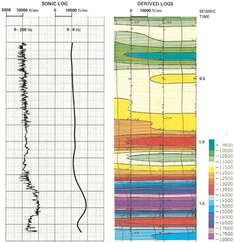
Fig. 8. Comparison of Low Frequency Components from Well Data with that Derived from Stacking Velocities
