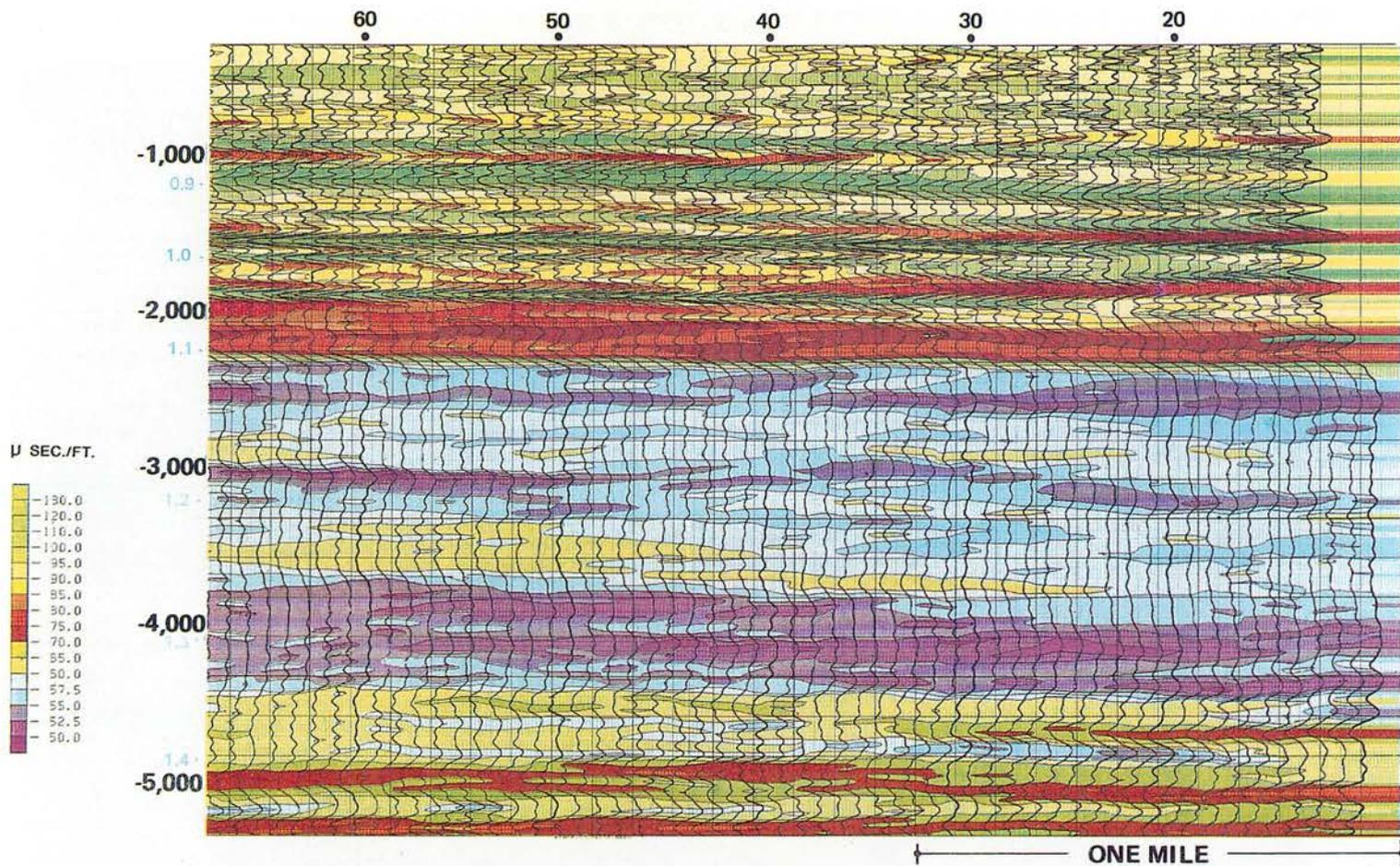
Fig. 12. SEISLOG Display of Seismic. Inversion of a window of the seismic data. Transit times have been contoured and colour coded as indicated by the colour bar to the left. Each trace is a synthetic sonic log. The unconformity separating clastics from Carbonates is clearly visible as a distinct colour change near 2000 ft. The reef is the irregular dark blue mass near 3000 ft. Both sections are uninterpreted, displaying the seismic data presentation after processing ready for interpretation.
