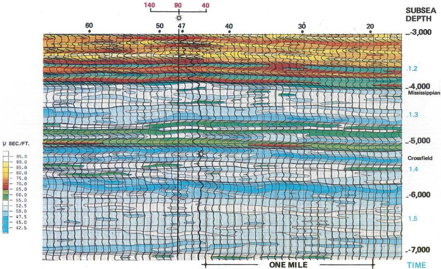
Fig. 16. A SEISLOG display of part of the seismic data shown in figure 15. The zone of interest is labelled Crossfield near -5250 feet.
