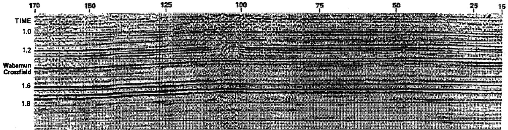
Fig. 15 Conventional Seismic Across Regional Carbonate. Seismic line across a gas field. Production is obtained from dolomitized porosity in an algal bank in Devonian carbonate section. The zone of interest is the Crossfield.
