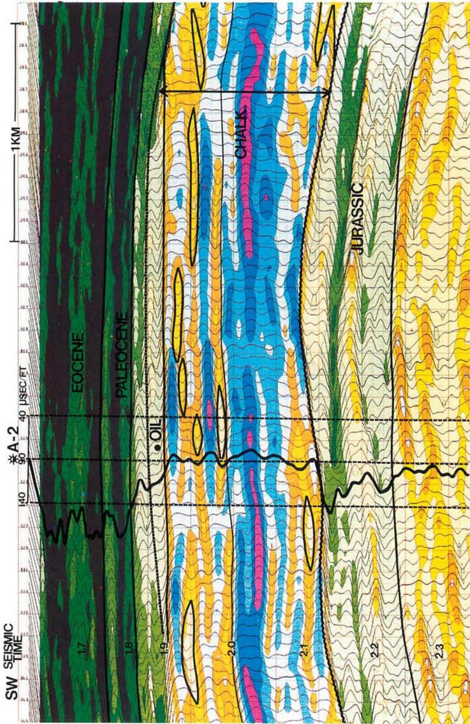
Fig. 19. SEISLOG Display at A-2, Arne Structure, North Sea
