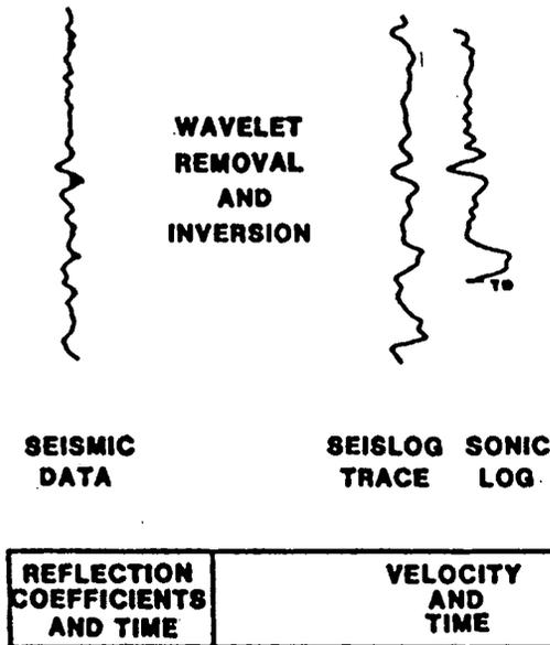
Fig. 4. Inverse Model. In the inverse model approximations of borehole sonic logs are constructed from seismic data after appropriate wavelet removal. These logs can be correlated with borehole sonic logs that have comparable bandwidth.
