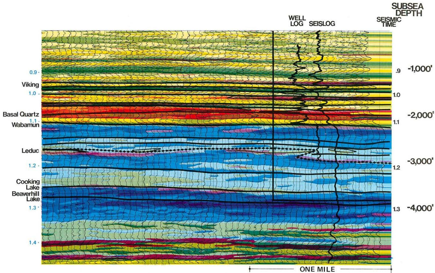
Fig. 13. Interpreted Depth SEISLOG Display of a Devonian Reef in Western Canada
