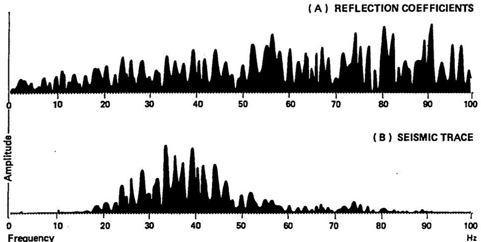
Fig. 5. Comparison of Amplitude Spectra from Well Data and Seismic
