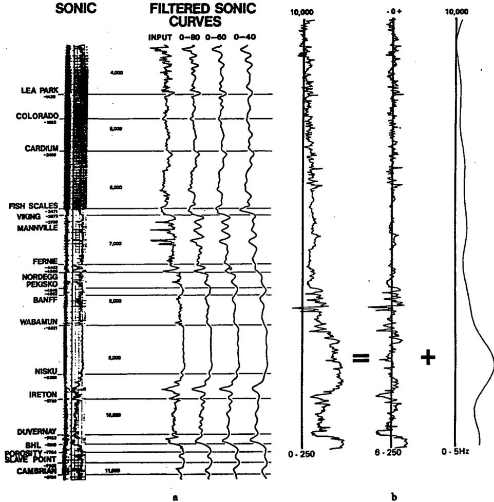
Fig. 6. Effect of Filters on Raw Sonic Data. (a) Loss of high frequency decreases resolution on sonic logs. (b) The basic velocity structure of a sonic log is provided by the very low frequencies, while the higher frequencies provide the detailed resolution.
