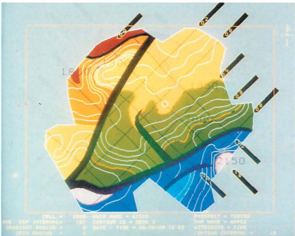
Fig. 18. Map by automatic contouring and finalized with colour and annotation.
