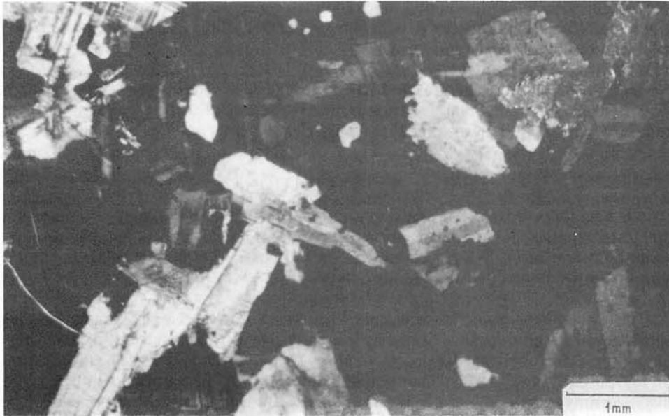
Fig. 3 Large poikilitic microcline grain (in extinction) with inclusions of muscovite, plagioclase and quartz.
