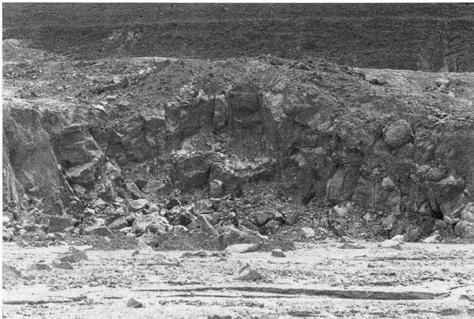
Plate 2. Inhomogeneous overburden due to differential pattern of weathering. Unweathered bedrock materials enveloped by highly weathered residual soil. (Taman Tun Abdul Razak, Ampang, Kuala Lumpur)
