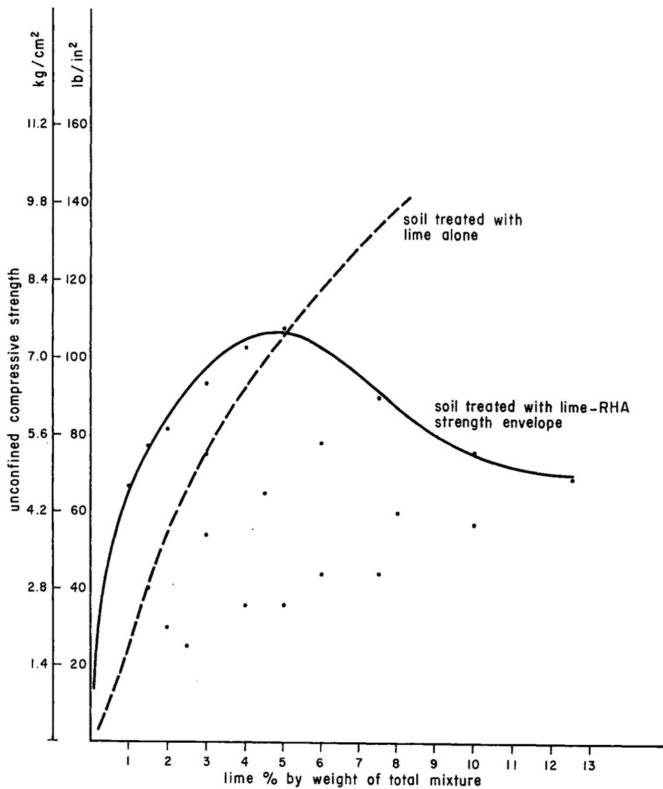
Fig. 4. Effect of RHA on optimum lime content for maximum strength (28-day curing)
