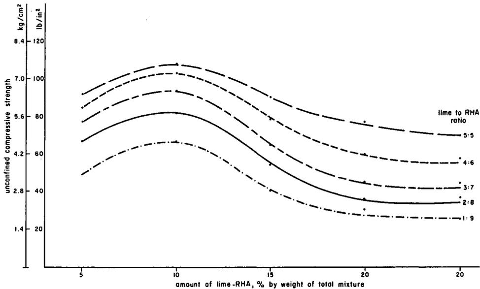
Fig. 3. Effect of amount of admixture on strength of lime-RHA stabilized soil. (28-day strength values)
