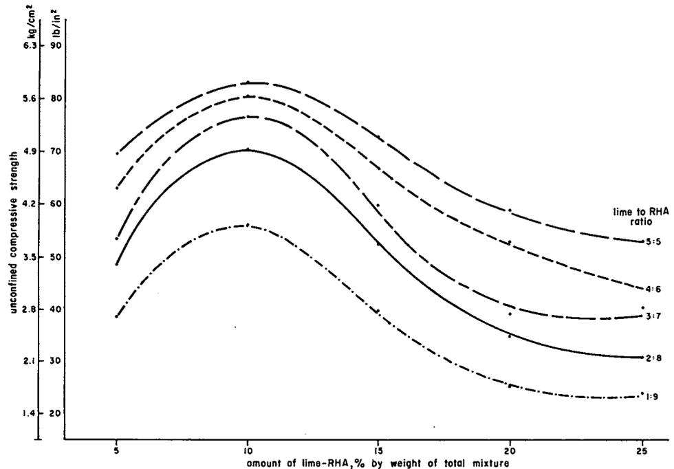
Fig. 2. Effect of amount of admixture on strength of lime-RHA stabilized soil (7-day strength values)
