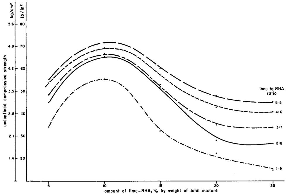
Fig. 1. Effect of amount of admixture on strength of lime-RHA stabilized soil (3-day strength values)
