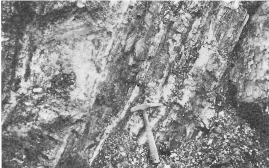
Plate 2. Weathered face, Nam Salu Open Cut, Kelapa Kampit Mine, Belitung, Indonesia; well bedded stanniferous lode, sulphides altered to iron oxides.
