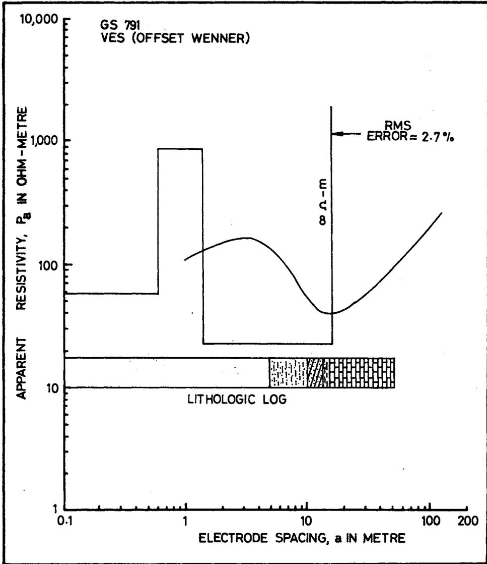
Figure 9: Interpretation of Vertical Electrical Sounding at GS 791
