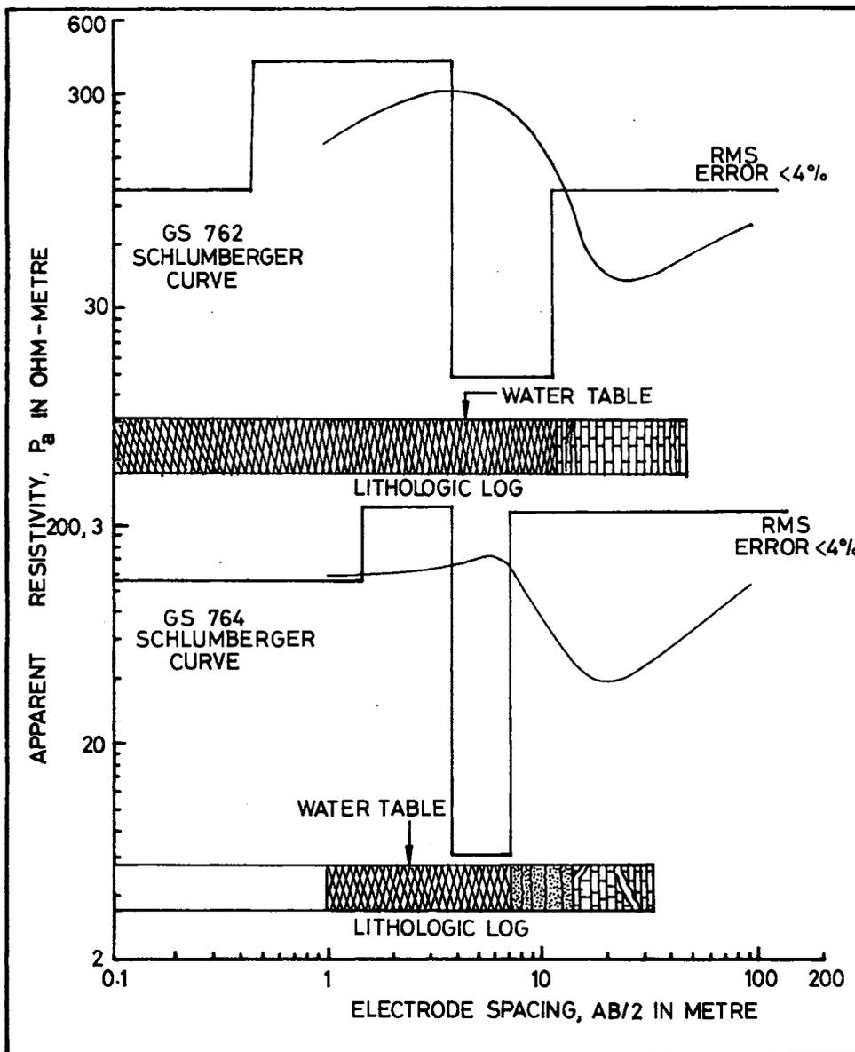
Figure 6: Interpretation of Vertical Electrical Sounding at 762 & 764
