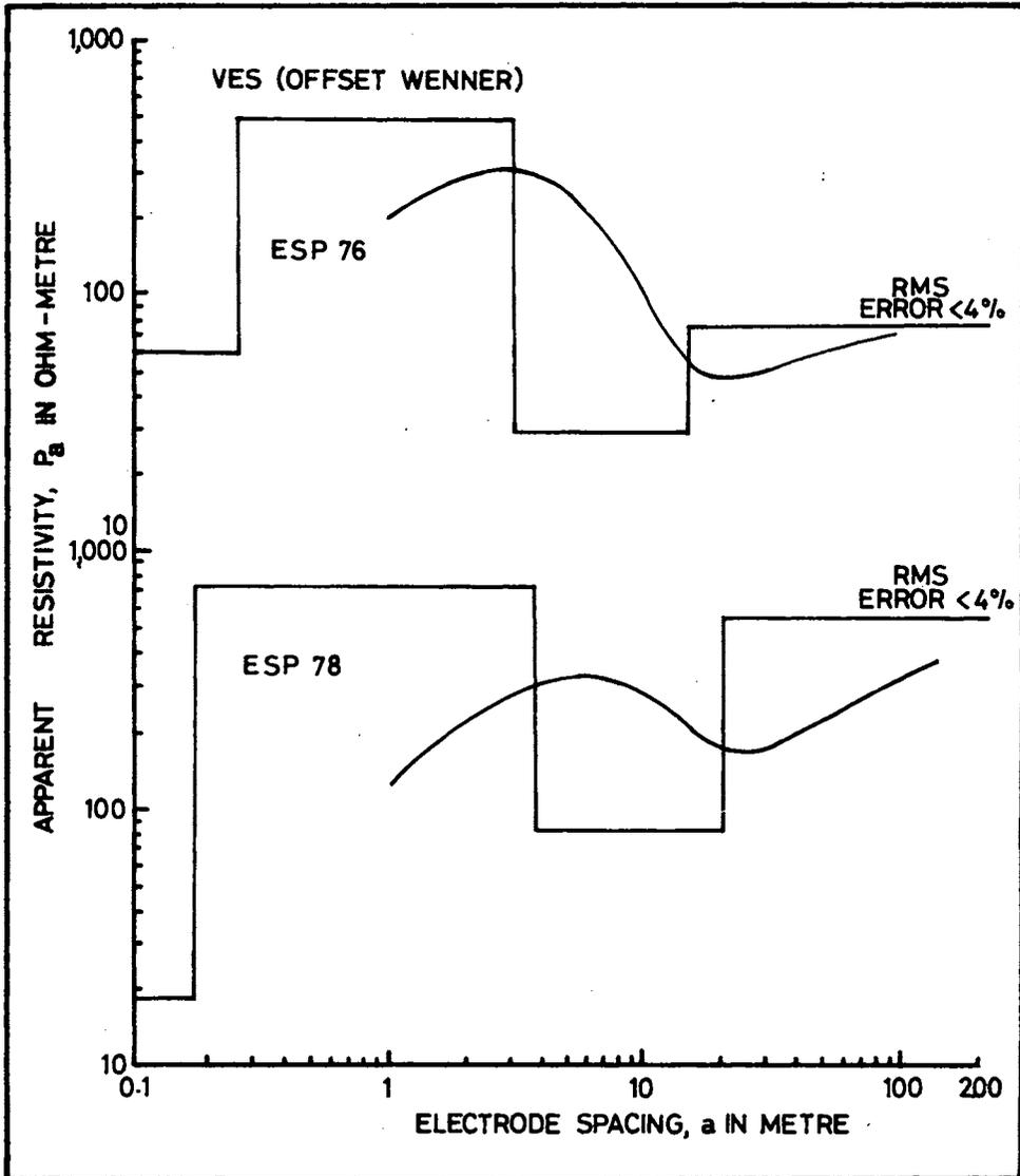
Figure 7 : Interpretation of Vertical Electrical Sounding at ESP 76 & 78
