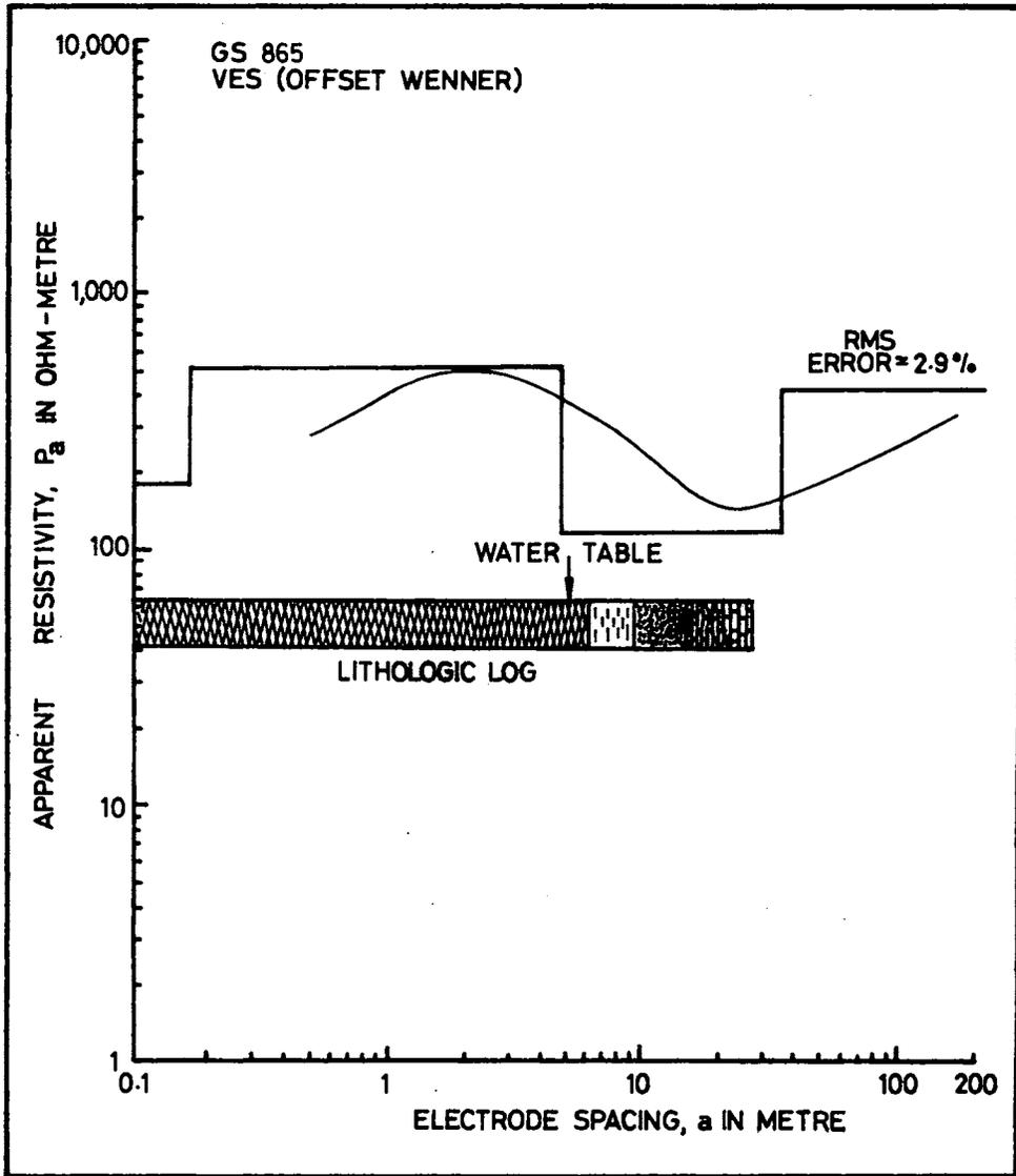
Figure 4 : Interpretation of Vertical Electrical Sounding (VES) at GS 865
