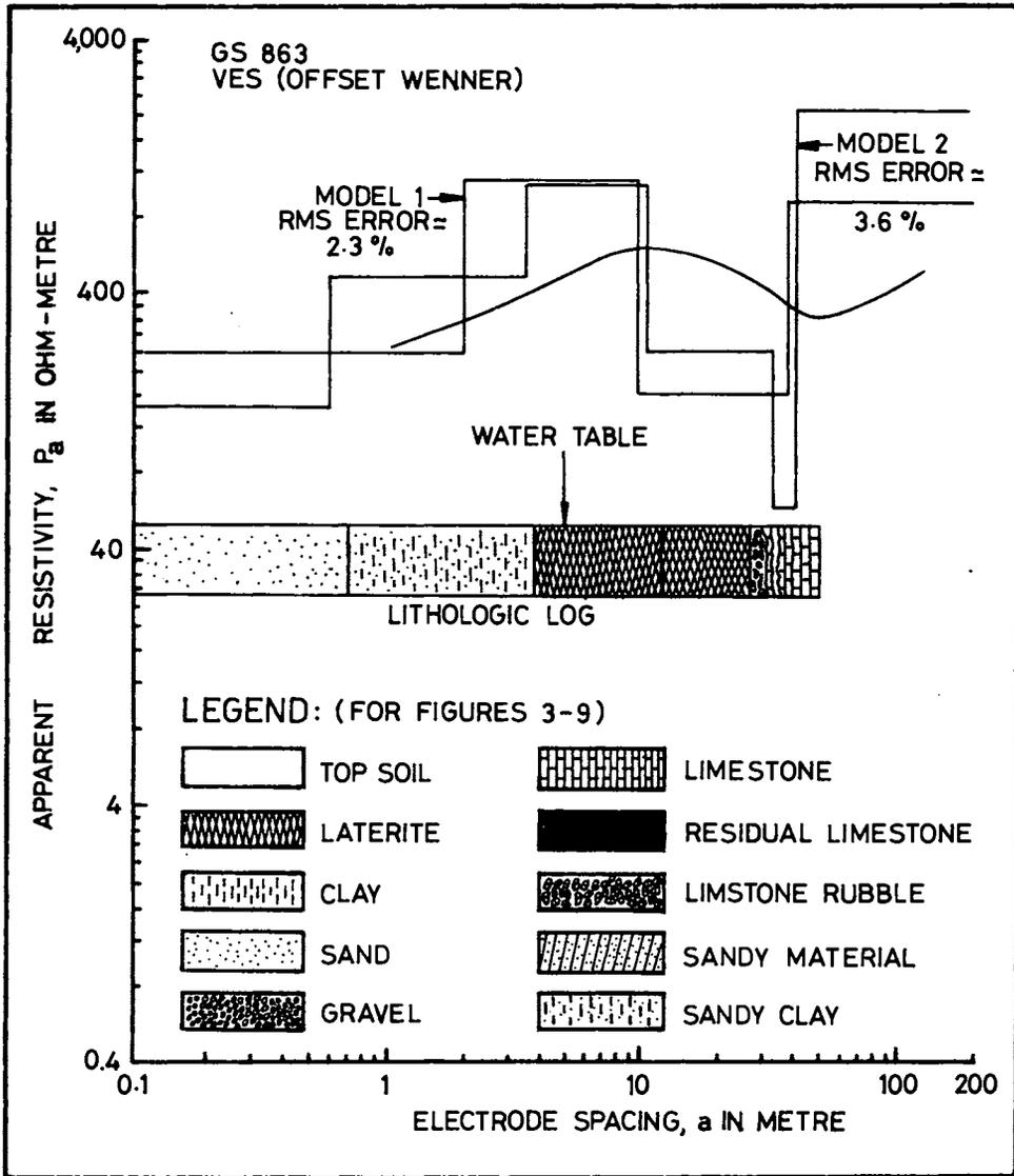
Figure 3 : Interpretation of Vertical Electrical Sounding (VES) at GS 863
