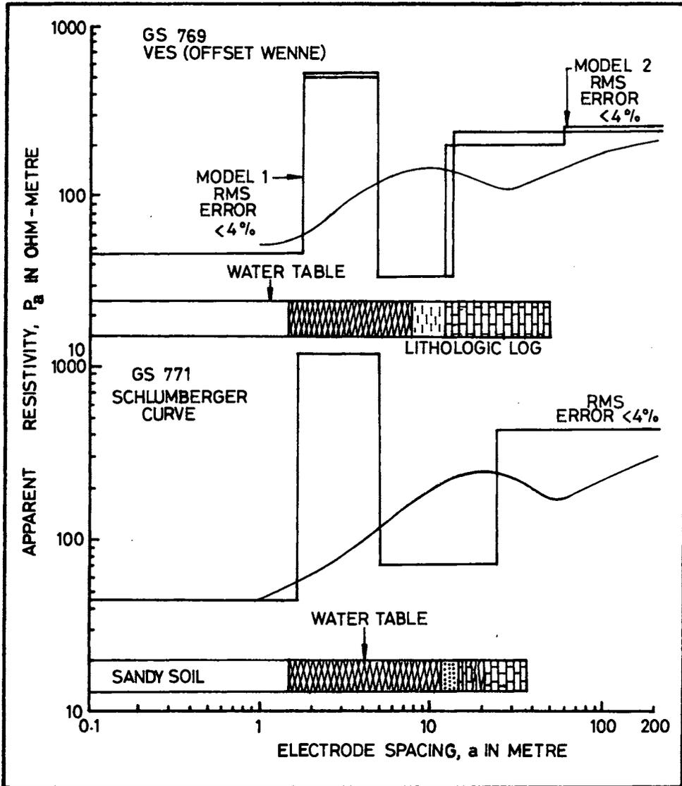
Figure 5: Interpretation of Vertical Electrical Sounding (VES) at GS 769 & 771
