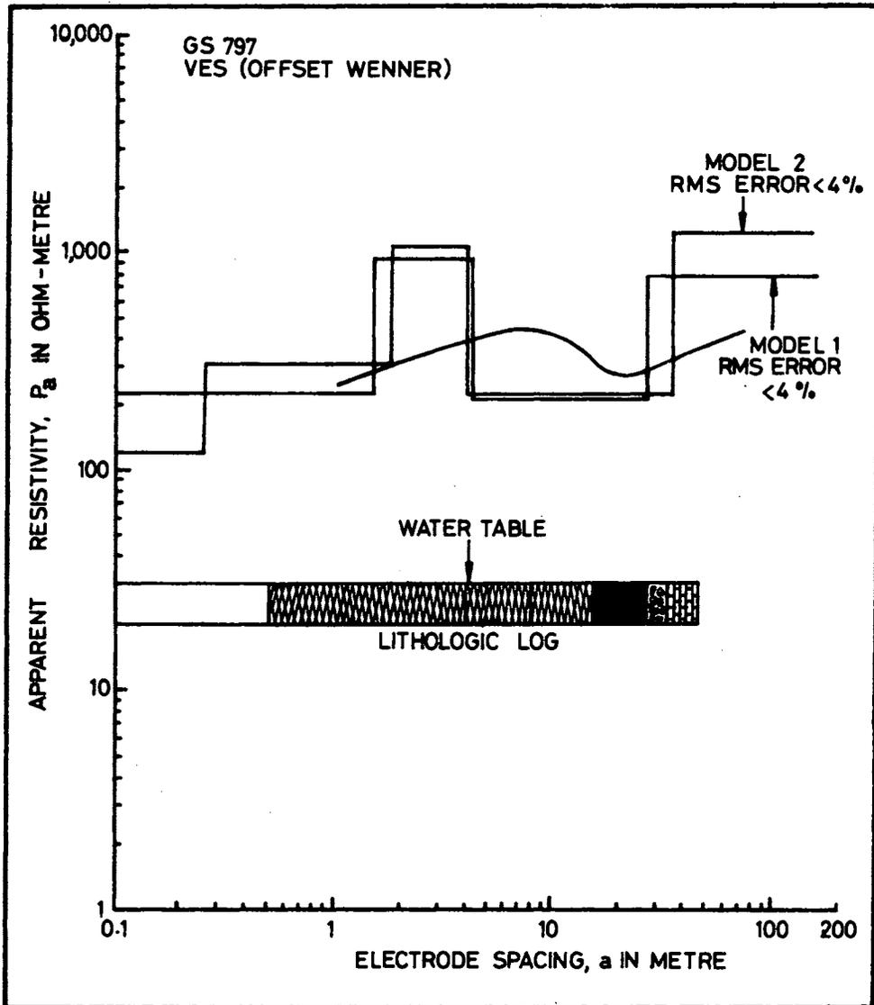
Figure 8 : Interpretation of Vertical Electrical Sounding at GS 797
