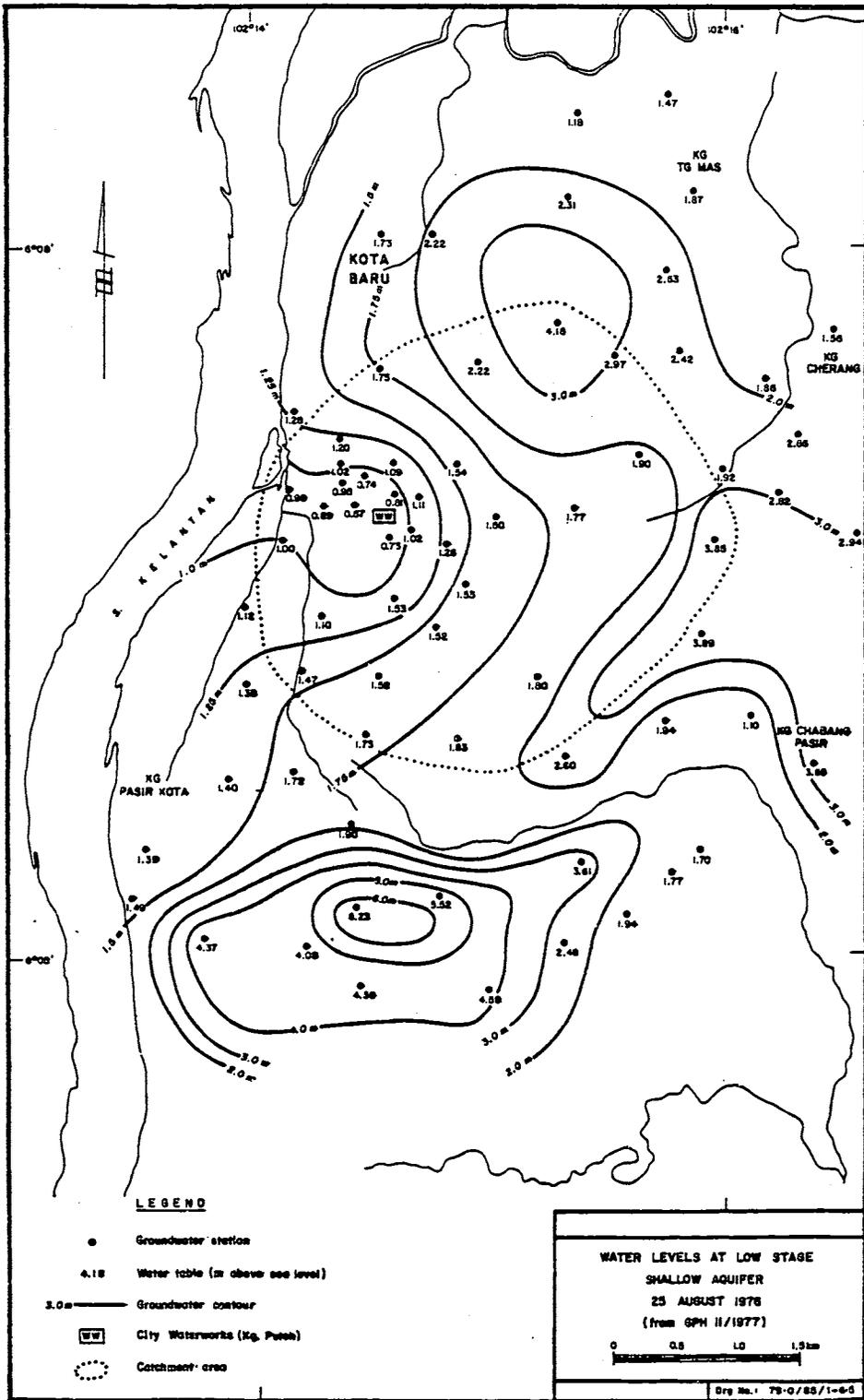
Figure 3 : Water levels at low stage, shallow aquifer, 25 August 1976 (from GPH II/1977)
