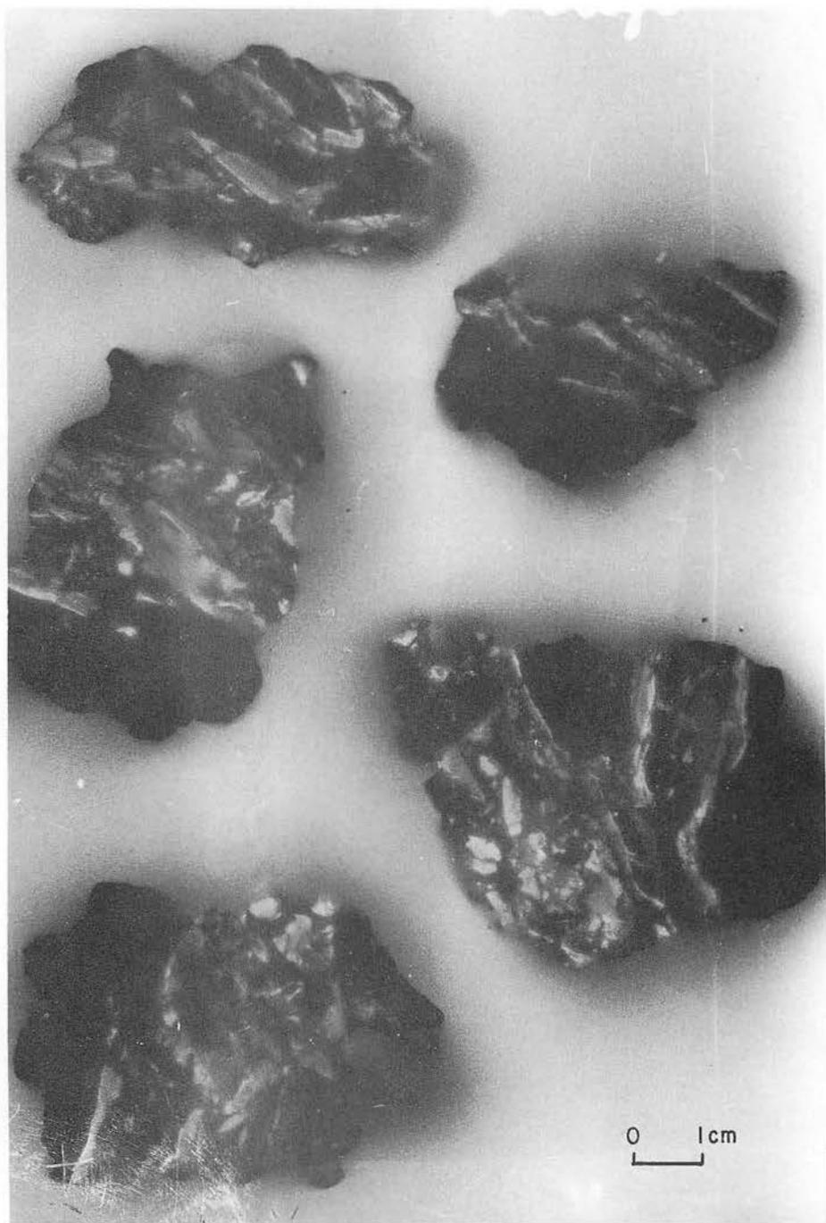
Plate 4. Printed autoradiographs of radioactive samples from locality B. Radioactive centres appear white, consisting of a mixture of uranium-bearing florencite and rhabdophane. (AMDEL Service Report GS 4333/83, 1983). Actual size. Specimen showed 760 ppm leacheable U.
