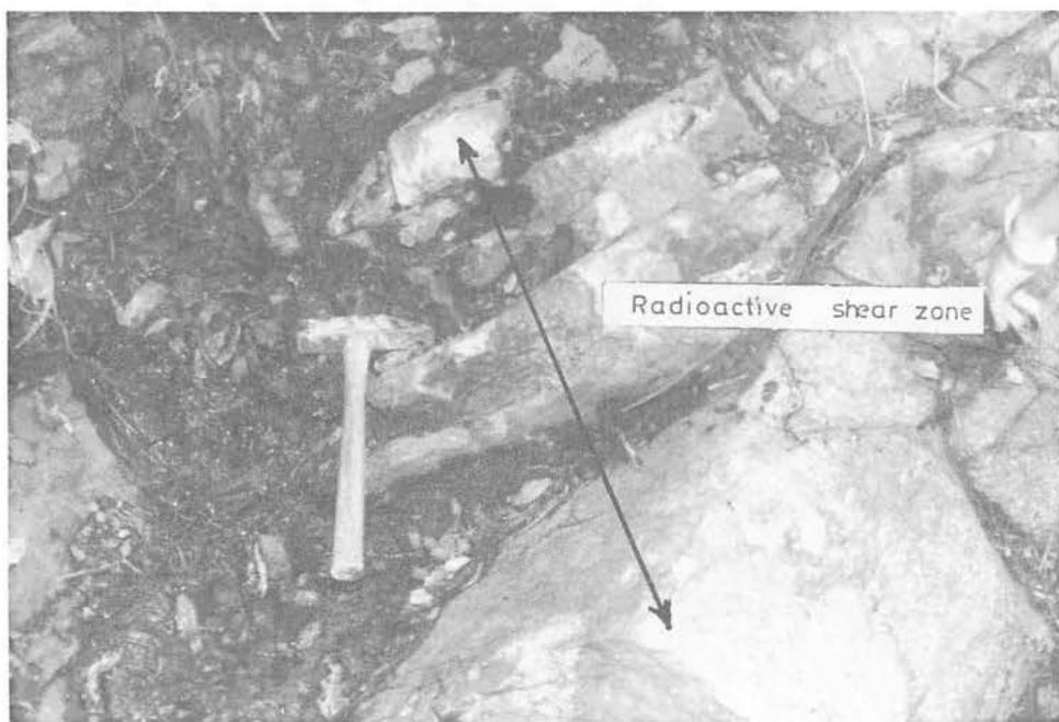
Plate 9. Radioactive shear zone in granite; total count readings range from 600-750 cps. Shear zone showed 308 ppm leachable U over 0.5 m (Locality C).
