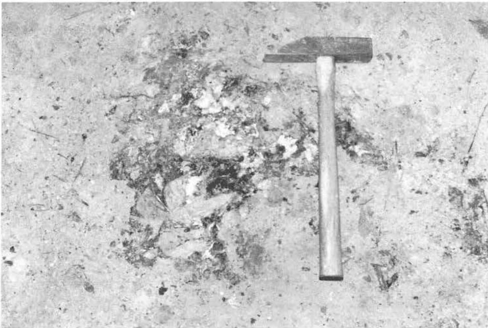
Plate 3. Close-up view of iron-stained radioactive showing (Locality B). Total counts range from 700-750 cps. Readings taken with Geometrics GR 101A Scintillometer.
