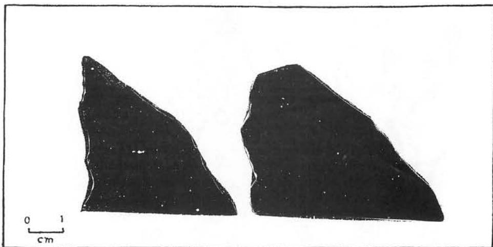
Plate 1. Printed autoradiographs of radioactive samples from locality A. Uraninite crystals measuring 15-50 $\mu$ m appear as white dots. Other minerals include chlorite, hematite and pyrite. (AMDEL Service Report GS 4333/83, 1983). Actual size. Specimen showed 277 ppm. leacheable U.
