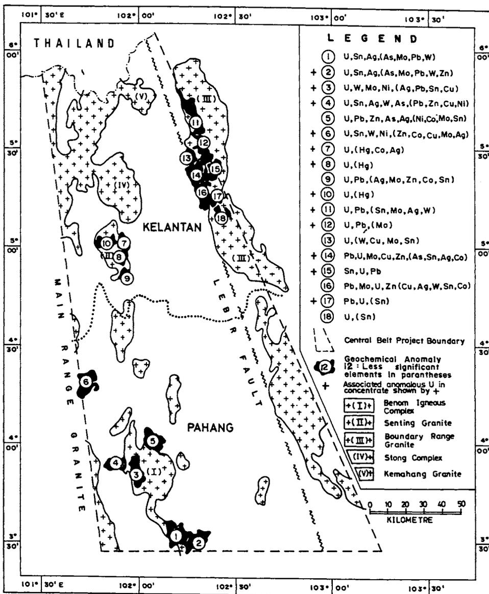
Fig. 6 Stream sediment anomalies with associated uranium highs (Data up to 1978).
