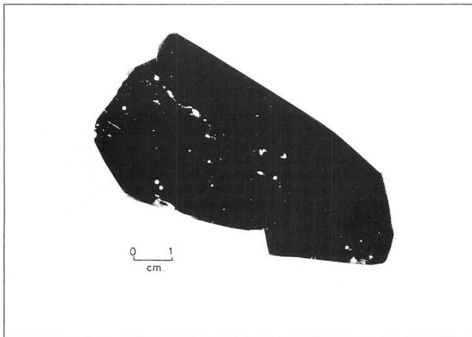
Plate 6. Printed autoradiograph of brecciated magnetite-rich granite 3505/UV/1A, from locality C. Radioactive centres appear as white spots, probably uraninite? Autoradiograph prepared locally at Kota Bharu, 5 days exposure, using ASA 400 ILFORD negative.
