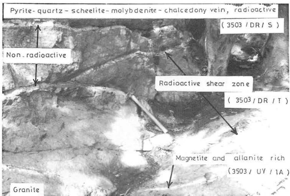
Plate 5. Radioactive vein and shear zone in granite, locality C. Vein gives 360-400 cps; shear zone shows 520-720 cps. Non-radioactive granite shows 200 cps. Background counts are 110 cps. All readings taken with Geometrics GR 101A Scintillometer. Specimens taken for autoradiography are indicated. Shear zone returned 105 ppm leachable U over 0.65 m.
