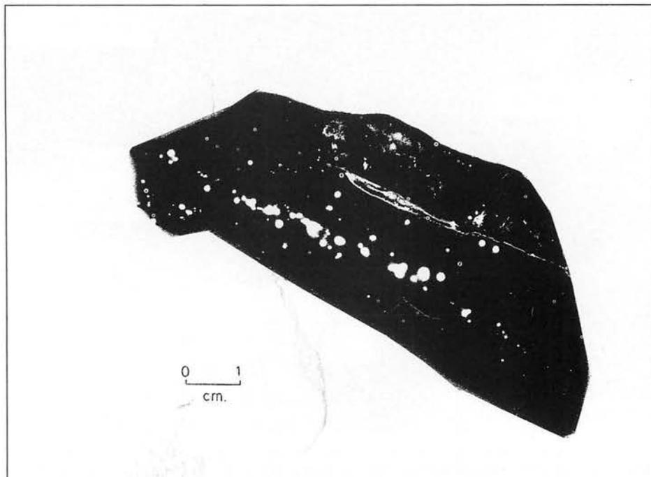
Plate 7. Printed autoradiograph of pyrite-quartz-scheelite-molybdenite-chalcedony vein 3505/DR/S, from locality C. Sample showed 1075 ppm leacheable U. White spots are radioactive centres. Autoradiograph prepared locally at Kota Bharu, 5 days exposure, using ASA 400 ILFORD negative.
