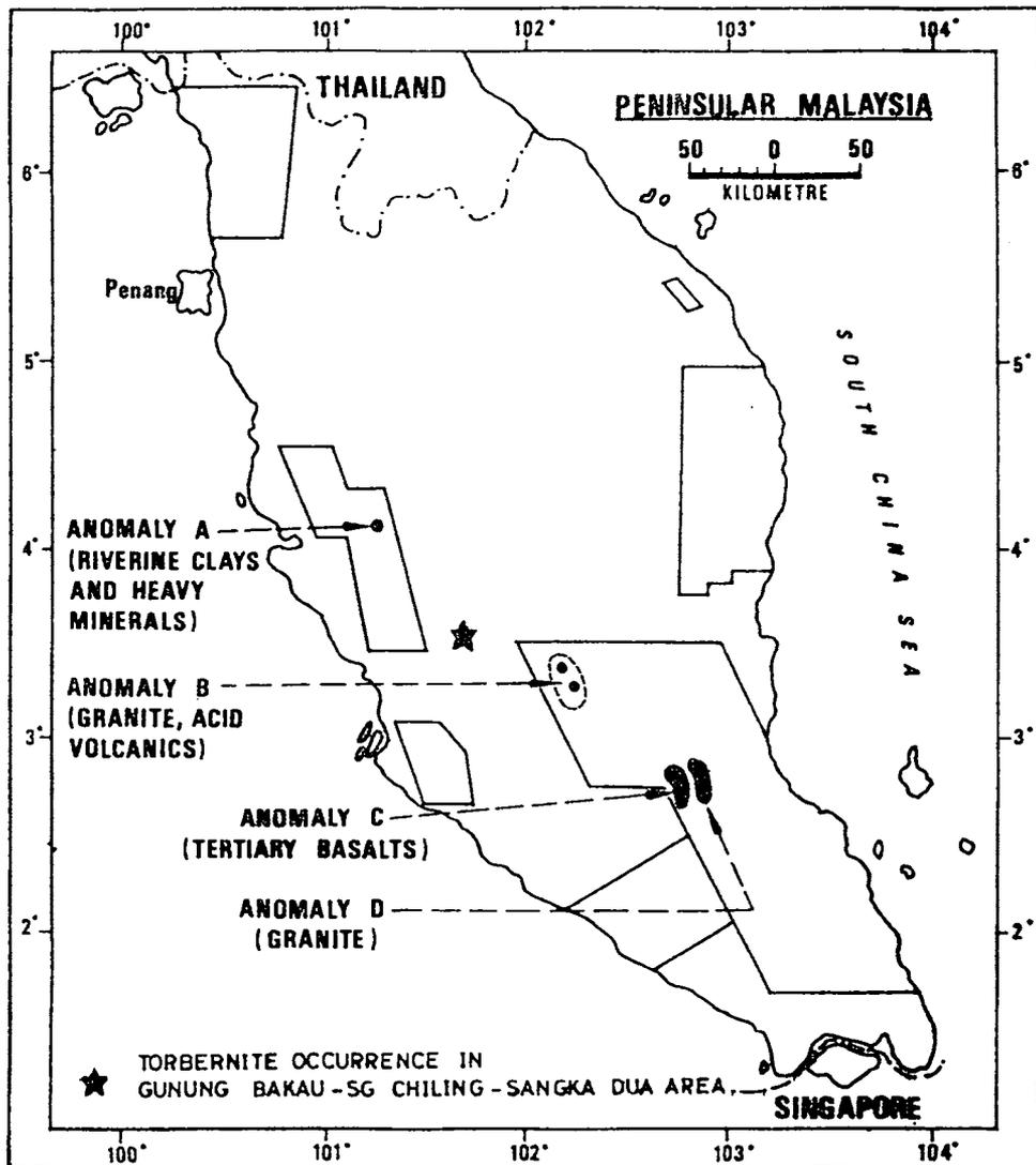
Fig. 1. 1956-57 Airborne areas showing some high radioactive anomalies (after AGOCS, 1958).
