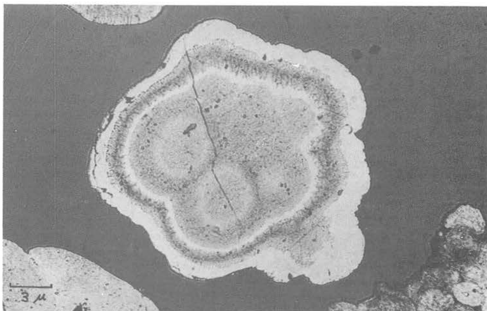
Fig. 12 A photomicrograph of a polished section of a galena nodule which has been etched to emphasise its zoning. Locality: Lenggang, Belitung.
