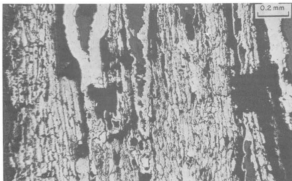
Fig. 9 A photomicrograph of a polished section of wood from Pengerang, South Johore, whose cell-walls have been locally distorted and even obliterated during the process of marcasitisation.
